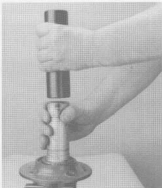
30. Coat the outer diameter of the input shaft bearing cover oil seal with Loctite #510. Install the oil seal on the front bearing cover with a bearing driver as shown. Install the input bearing race in the front bearing cover with the proper bearing driver.
