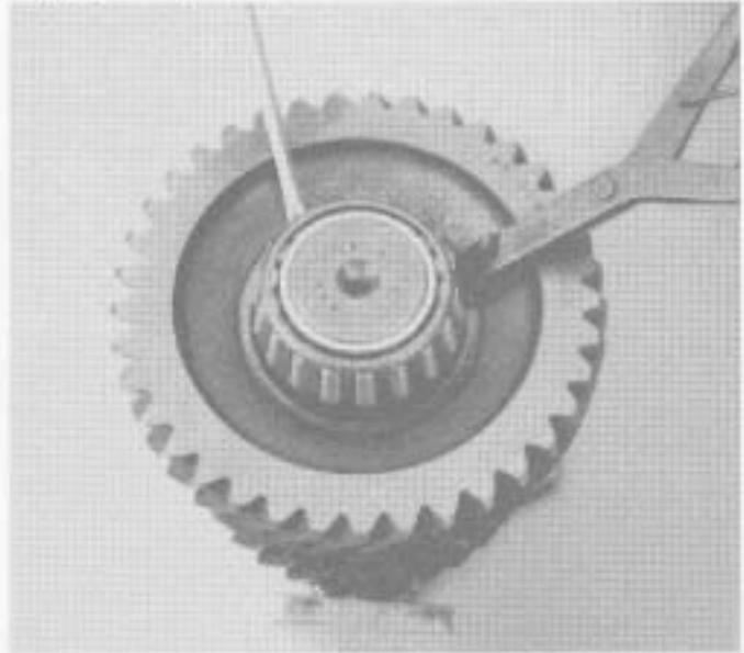
9. Use a screwdriver and snap ring pliers to move the snap ring out of snap ring groove and against the bearing back.
