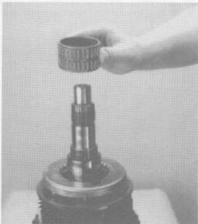
17. Install mainshaft 3rd speed gear bearing.
