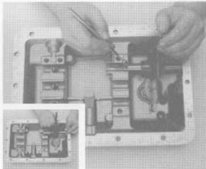
8. Remove the 1st-reverse lock pin from the 1st-reverse shift yoke assembly. Remove the 1st-reverse shift yoke (inset).
