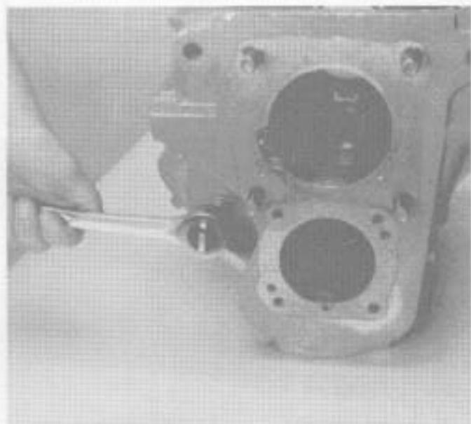
4. Remove the reverse idler retaining capscrew and the retainer.
