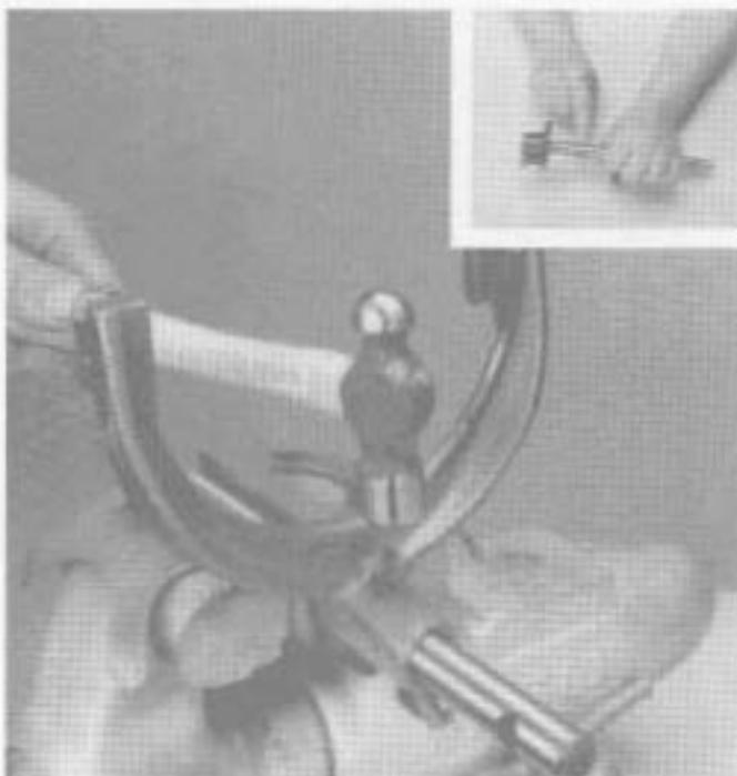
4. If shift blocks or shift yokes were removed, align shift yoke or block with alignment hole in the shift bar and insert lock pin.
