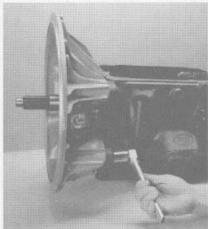
1. Position the transmission as shown. Place the clutch housing on the transmission case. Install the four retaining bolts and tighten to the recommended torque.
