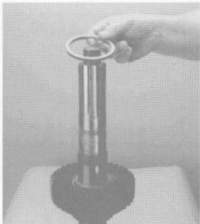
4. Install 2nd gear split washer retainer ring.
