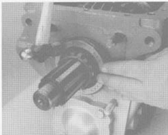
**33.** Install the main shaft rear outer bearing race in the output shaft bearing bore.
