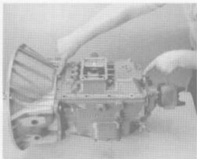
2. Apply Loctite #262 to threads of capscrews. Install two capscrews into shift bar housing alignment holes and tighten to the recommended torque.
