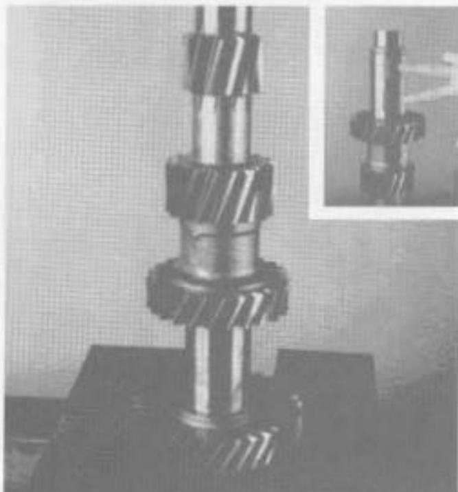
1. Install 4th and 5th speed gear keys in the countershaft keyways (inset). Align 4th speed countershaft gear keyway to shaft key. Press 4th gear on the countershaft, long hub to shaft front.
