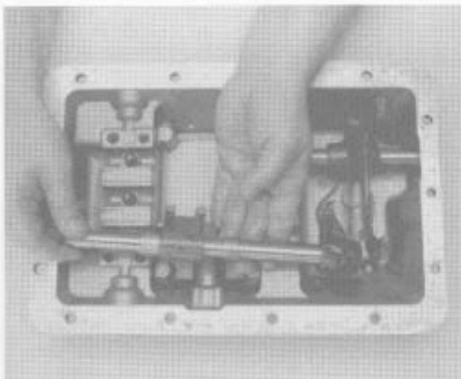
6. Remove 1st-reverse bar assembly. If necessary remove the front spacer from 1st-reverse shift bar (inset).
