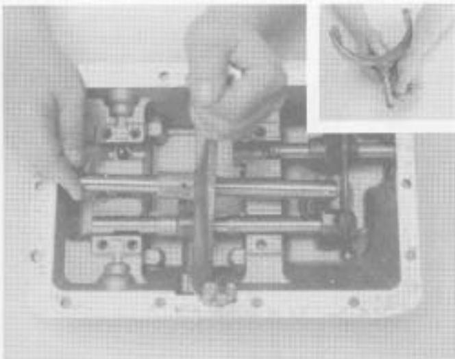
5. Remove 2nd-3rd yoke assembly and interlock pin (inset).
