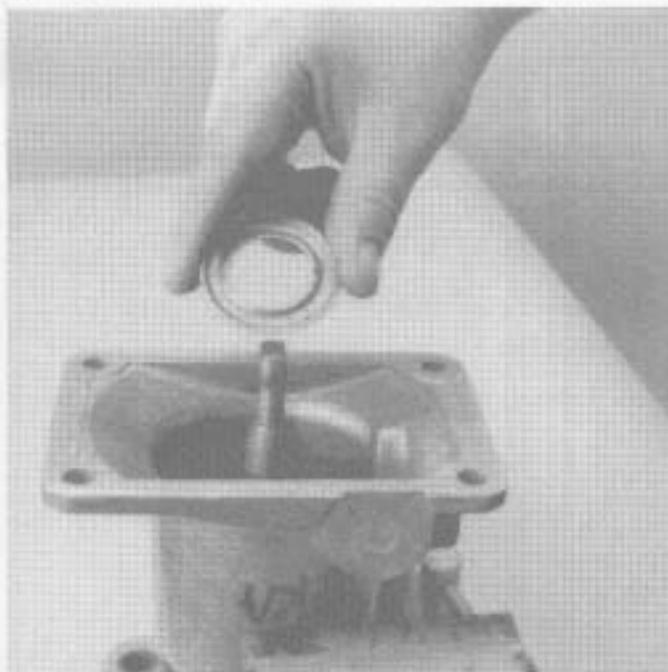
2. Position gearshift lever in housing with the spade pins in the lever ball slot and install the tension spring washer over the ball, dished side up.
