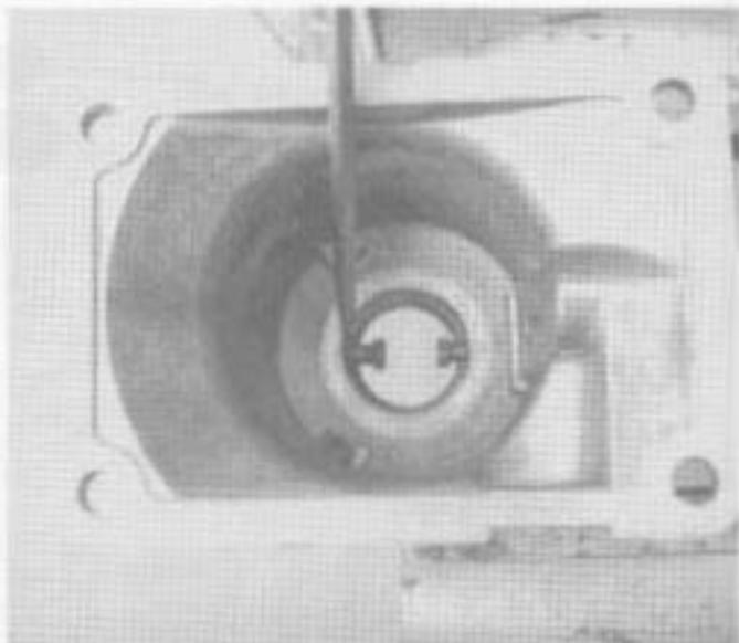
5. Remove the spade pins from housing bore.
