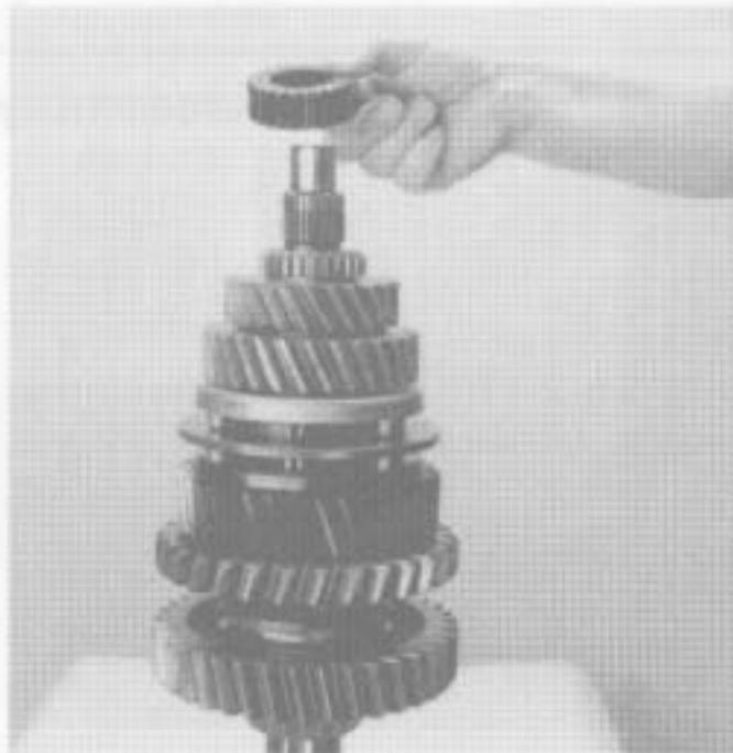
6. Remove 4th-5th speed clutch hub.
