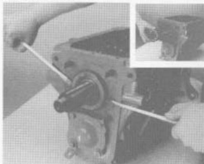
2. Remove speedometer drive gear (inset). Tap on the front of the main shaft to move the mainshaft rearward about 1/4". Use pry bars to remove the rear bearing cup and locating snap ring.
