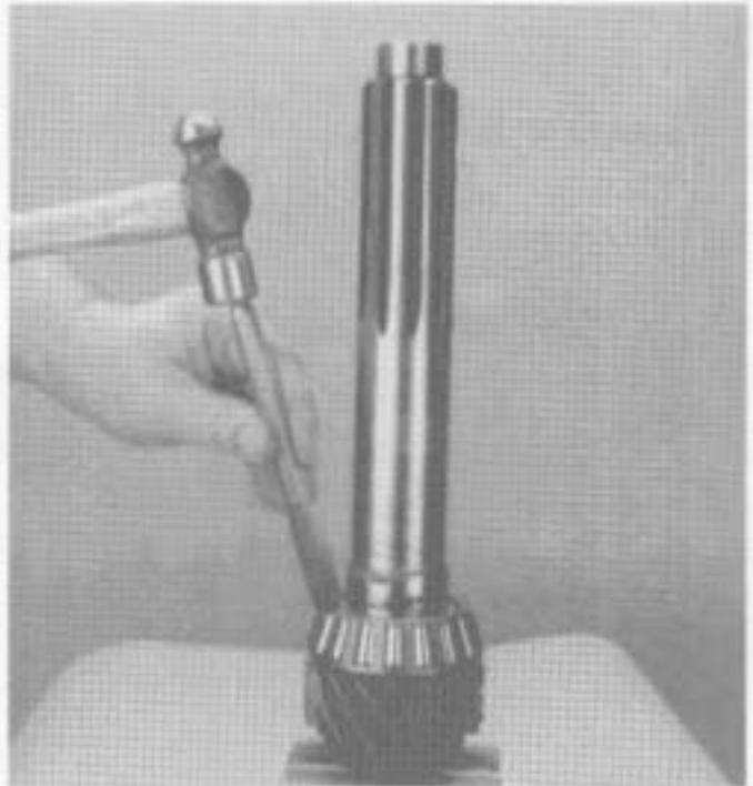
5. Use a chisel to remove the bearing cage and rollers. Install bearing puller and remove the bearing race from the input shaft.
