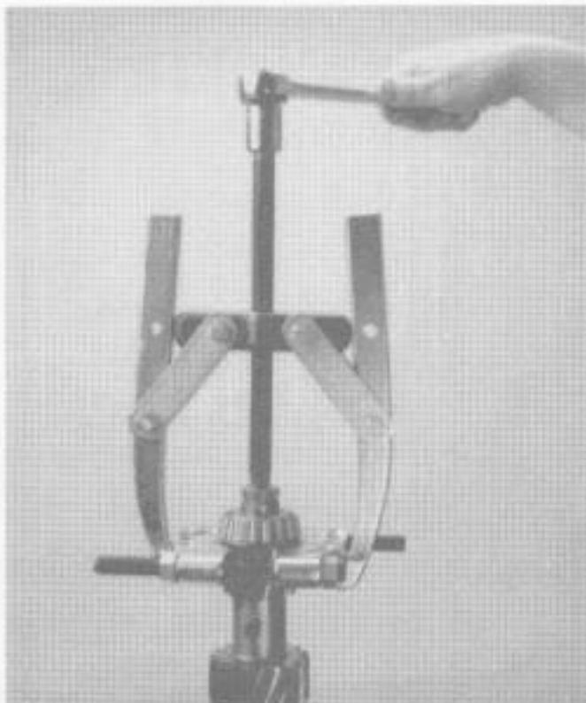
8. Position gear puller and clamp behind the rear countershaft bearing and remove the bearing.
