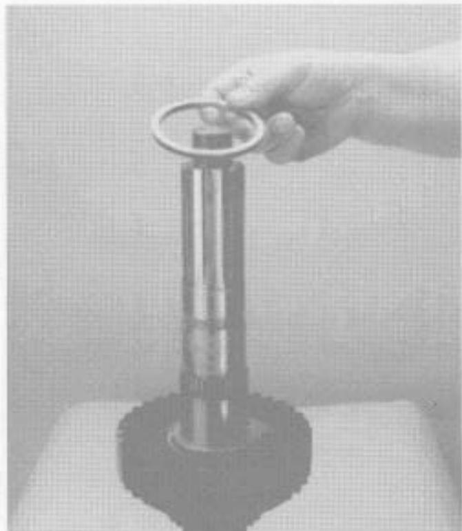
25. Remove 2nd gear split washer retainer ring.
