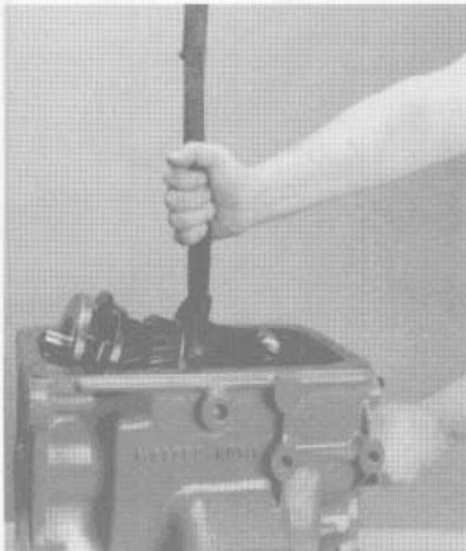
3. Wrap a sling or rope around the 2nd-3rd synchronizer. Use a hoist to remove the mainshaft assembly from the transmission case.
