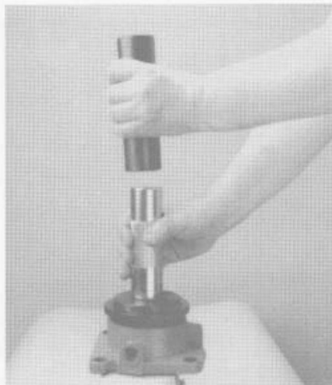
**34.** If a new oil seal is required, install using a flanged driver. Coat the oil seal outer diameter with Loctite #510.
