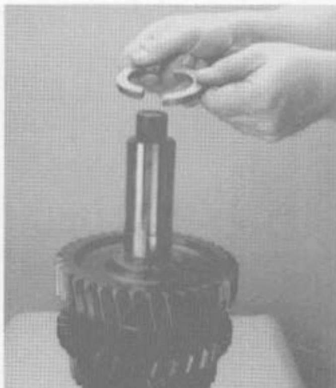
17. Remove the 1st gear split washer.
