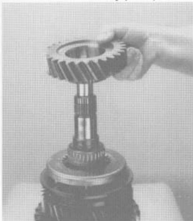
11. Remove the 3rd speed gear.
