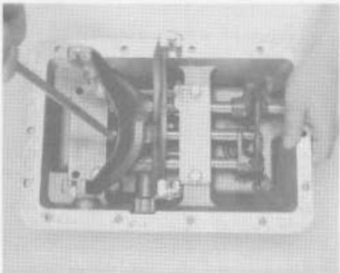
2. Lay the shift bar housing on the work bench. Remove two capscrews as shown and shift 4th-5th yoke assembly into 4th speed position with a screwdriver.
