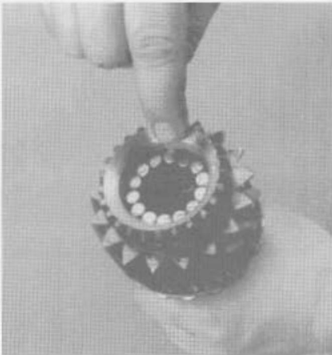
4. If necessary, remove the 14 roller bearings from the main drive gear bearing pocket.
