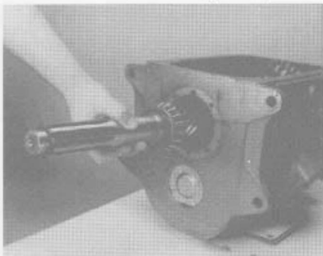
29. Install the input shaft by aligning clutching teeth on drive gear with teeth in mainshaft 5th speed synchronizer cup.
