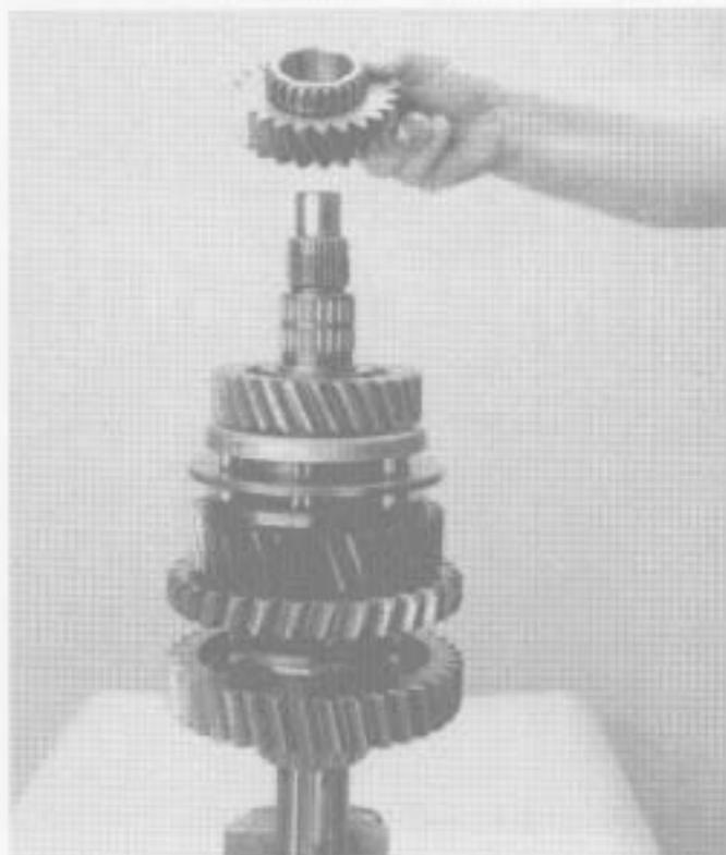
7. Remove the 4th speed gear.
