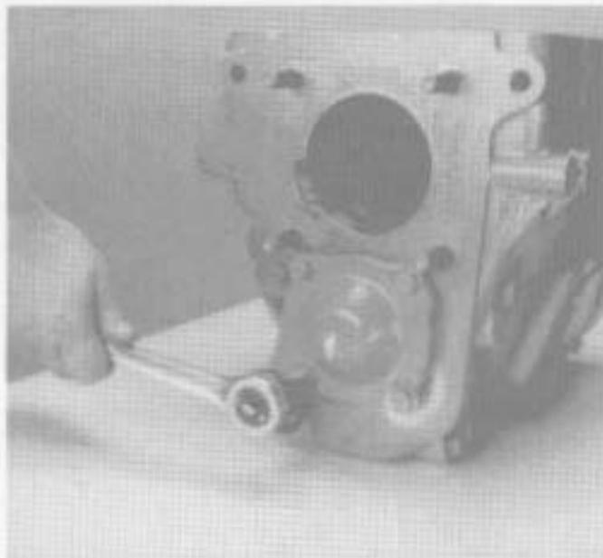
1. Remove the four cap screws and the countershaft rear bearing cover and gasket.
