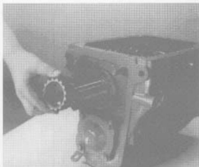
32. Install the speedometer drive gear or rotor on the output shaft.
