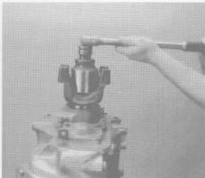
**37.** Place transmission in a vertical position as shown. Install yoke and nut. Tighten the yoke nut to recommended torque. Rotate the input shaft six times in each direction to seat the bearings and races.
