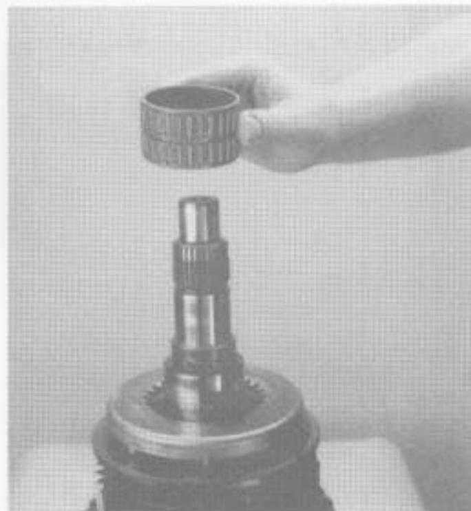
12. Remove the 3rd gear bearing.
