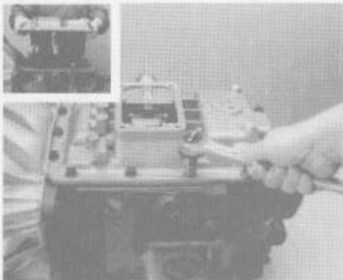
1. Shift the transmission into neutral position, remove the capscrews, and lift the shift bar housing and gasket from the case (inset).
