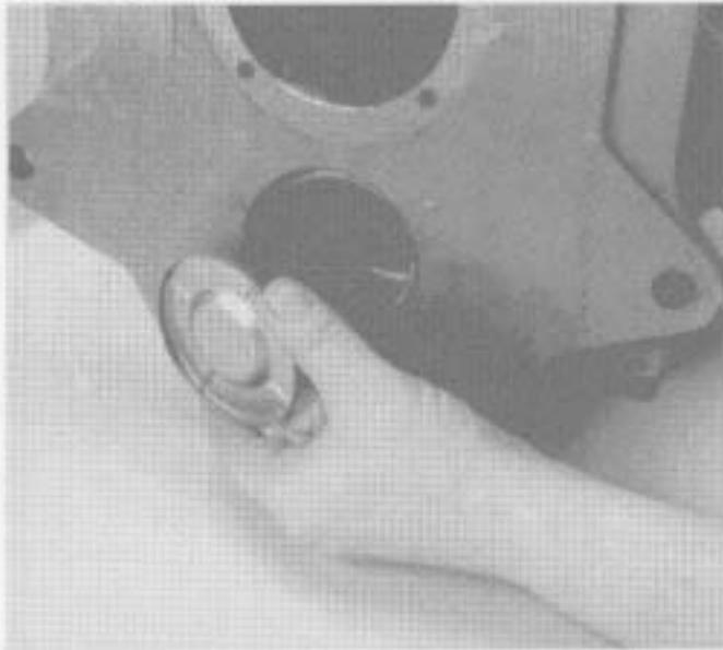
7. If the countershaft front bearing race is to be replaced, drive the bore plug through the front of the transmission and drive the race to the rear toward the case's inside.
