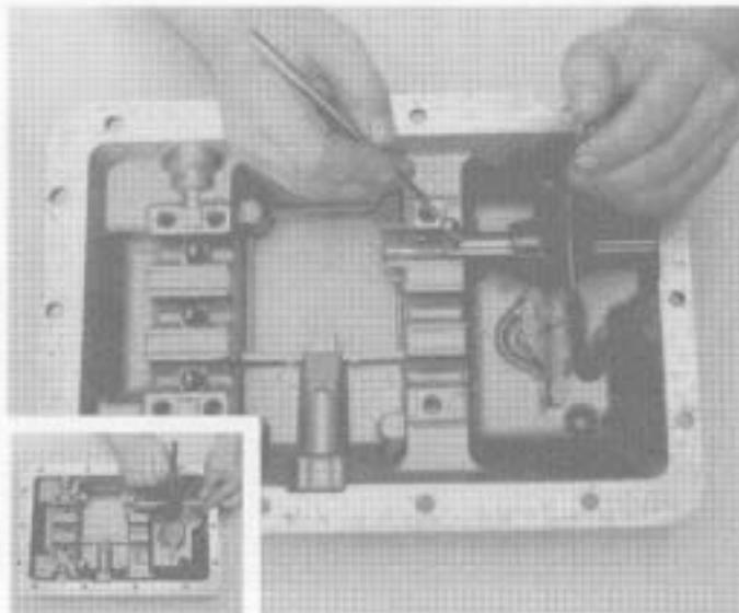
7. Position 1st-reverse yoke assembly in the shift bar housing (inset). Install the 1st-reverse lock pin in the yoke assembly.
