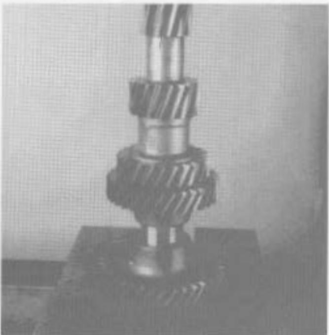
2. Press 5th speed countershaft gear on, long hub to shaft rear.
