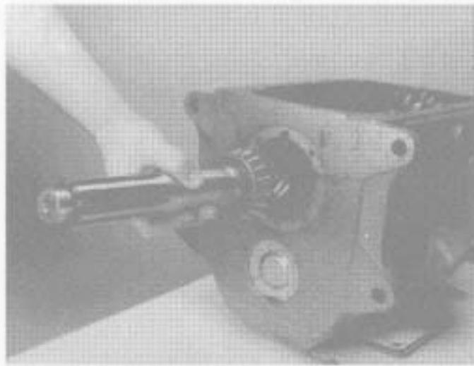
2. Remove the input shaft assembly from the transmission.
