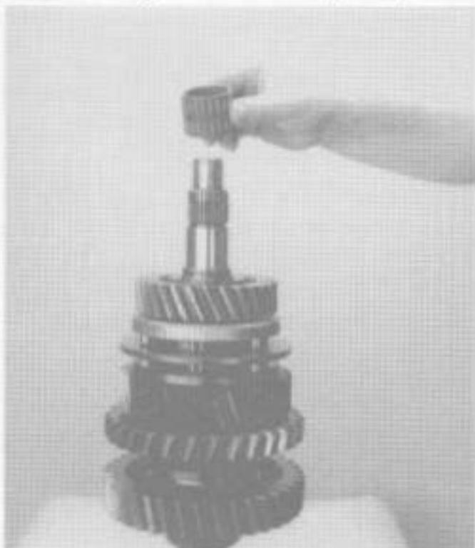
21. Install mainshaft 4th gear bearing.
