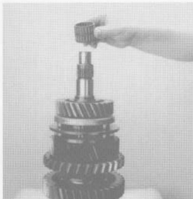
8. Remove 4th gear bearing.
