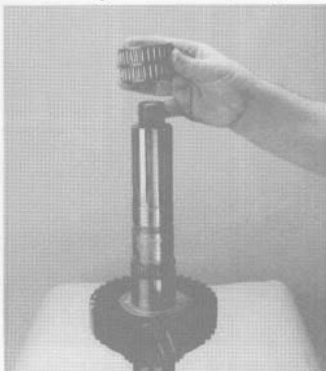
5. Install mainshaft reverse gear bearing.
