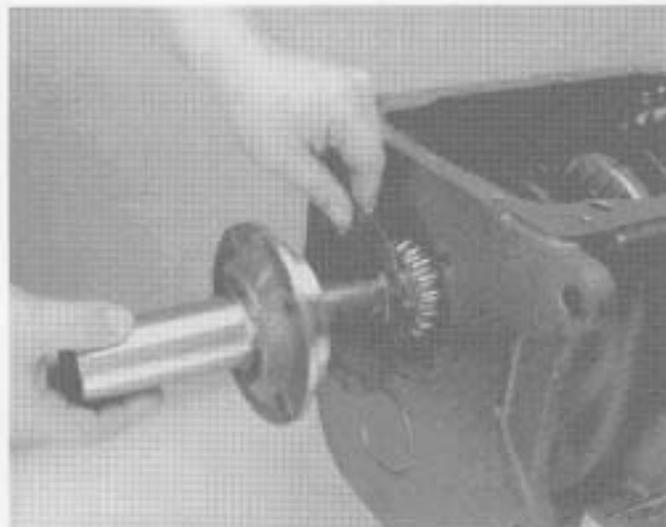
31. Install input shaft bearing cover, gasket, and cap screws. The front bearing cover lubrication oil groove must be at the top. Apply Loctite #262 to threads of cap screws and tighten to recommended torque.
