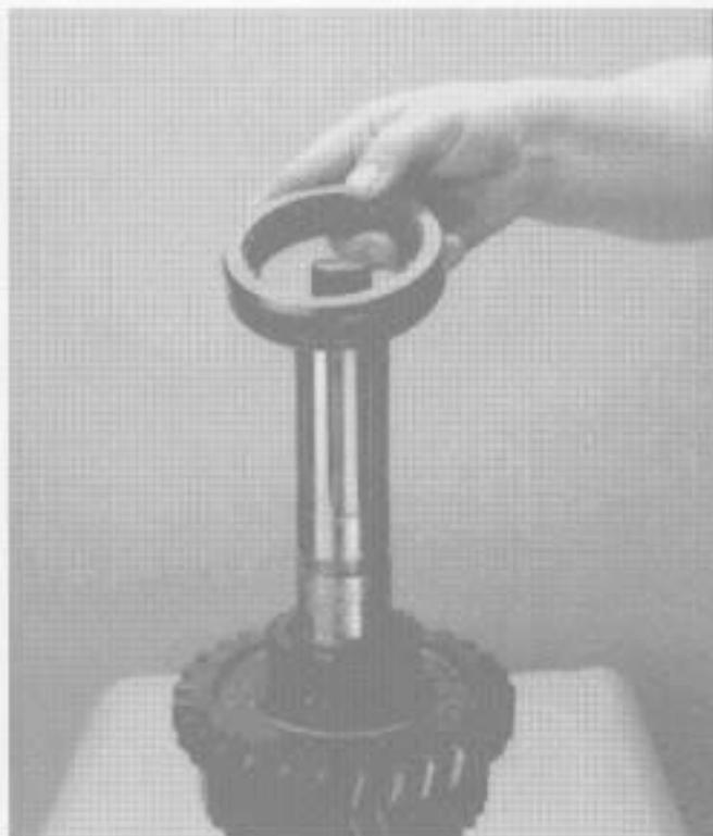
21. Remove the 1st-reverse sliding clutch.
