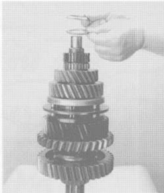
5. Remove the thrust bearing and bearing race.
