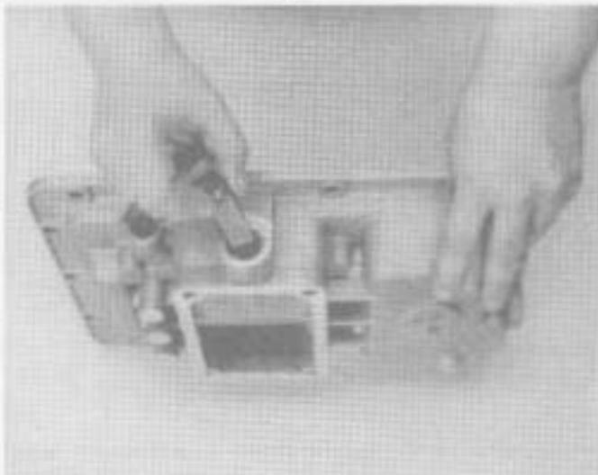
1. Place the shift bar housing on its side as shown and install the reverse plunger.
