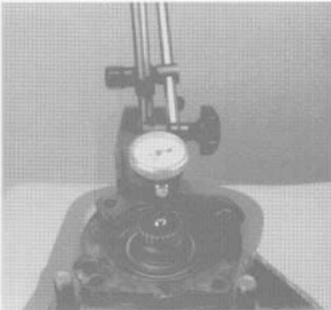
13. Rotate the countershaft to seat the bearings and races. Position the dial indicator as shown, lift the countershaft with a screwdriver to measure the end play. End play must be set at .002-.008 (0.05-0.20 mm). Add shims for more end play and remove shims for less end play.
