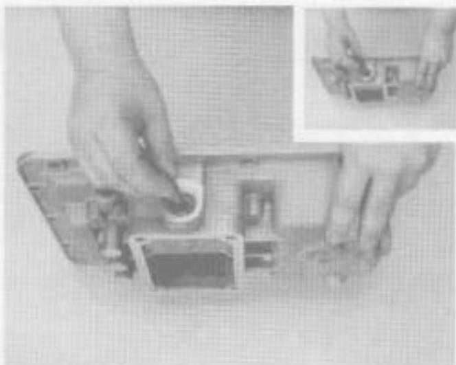
2. Install the reverse plunger spring (inset), and the reverse plunger stop.
