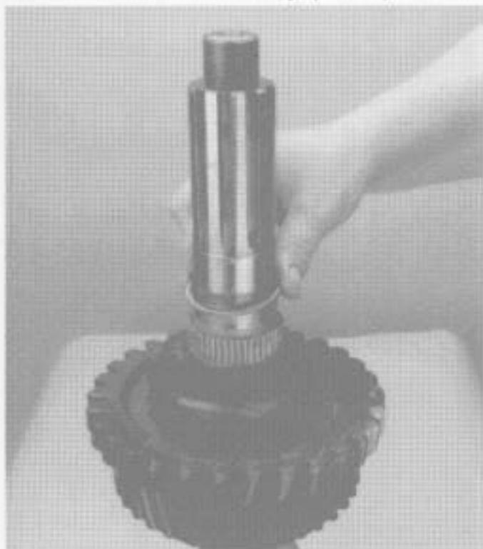
19. Remove the bearing rollers and spacers.
