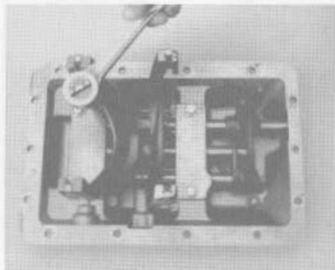
12. Install the remaining two capscrews and tighten capscrews to recommended torque.
