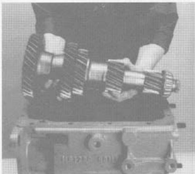
3. Move the countershaft assembly to the rear and lift it from the transmission case.
