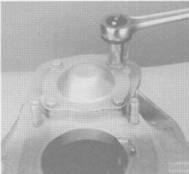
14. Install the countershaft rear bearing cover and gasket. Coat capscrew threads with Loctite #262 and tighten to the recommended torque.
