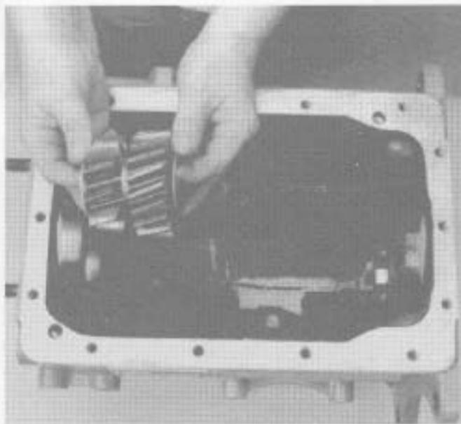
6. Remove the reverse idler bearings, spacer, and thrust washers.
