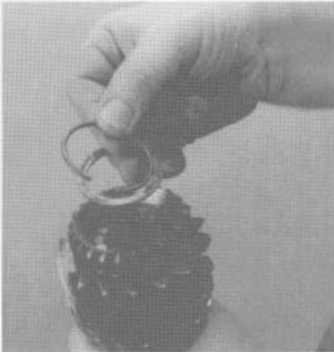
3. If necessary, remove the retention snap ring and the bearing retention ring.
