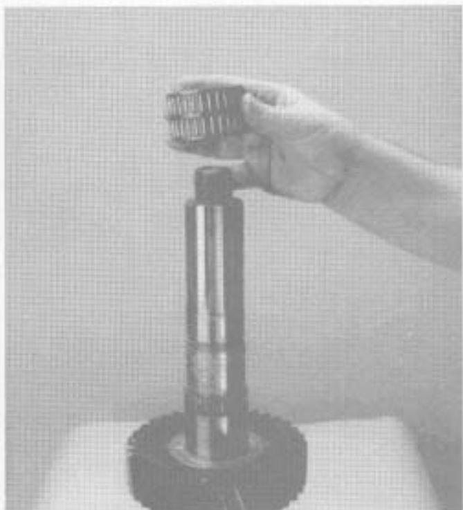
24. Remove the reverse gear bearing.
