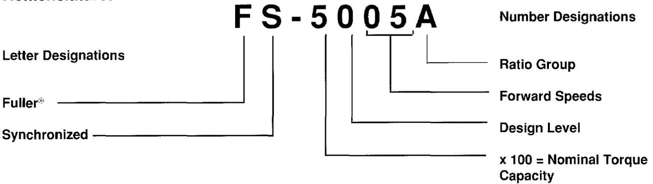
**IMPORTANT:** All Eaton Fuller Transmissions are identified by the model and serial number. This information is stamped on the transmission identification tag and affixed to the case.
