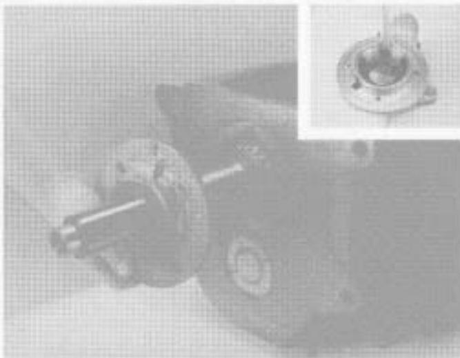
1. Remove the four capscrews from the front bearing cover and remove the cover and shims. The front bearing cover shims can come off with the front bearing cover. If necessary, remove the oil seal from the cover (inset).
