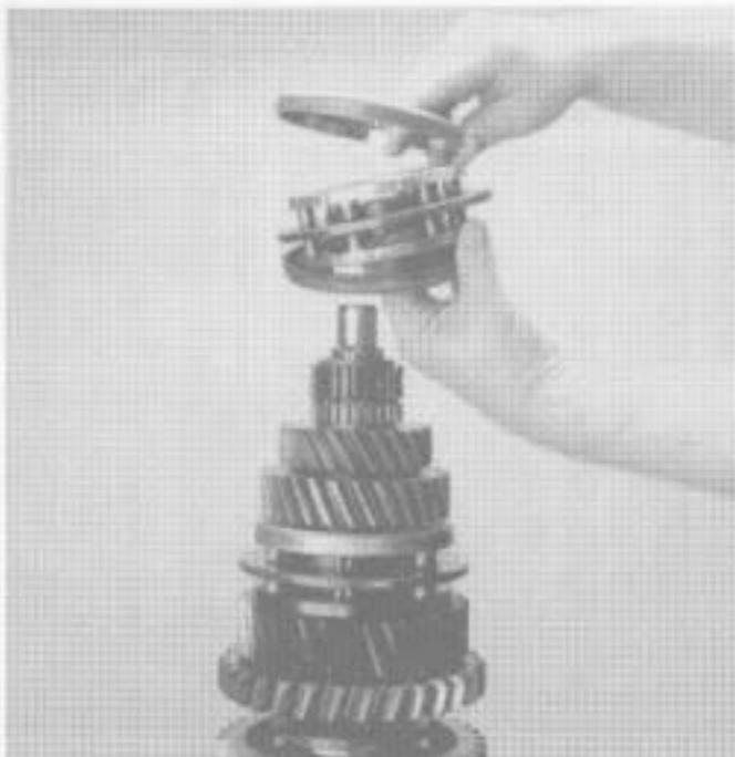
4. Install the mainshaft assembly in a vise equipped with soft jaws or wood, shaft front facing up. Remove the 4th-5th speed synchronizer and cups.
