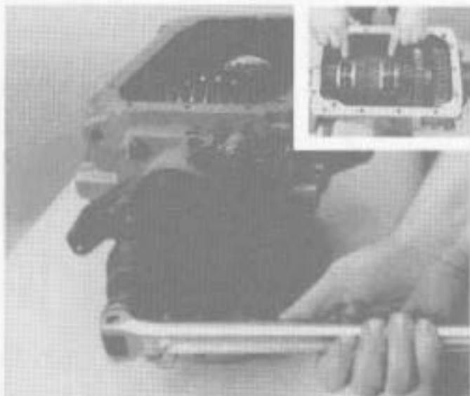
1. Lock the transmission by engaging two mainshaft gears as shown (inset). Use a large breaker bar to turn the retaining nut from the output shaft.
