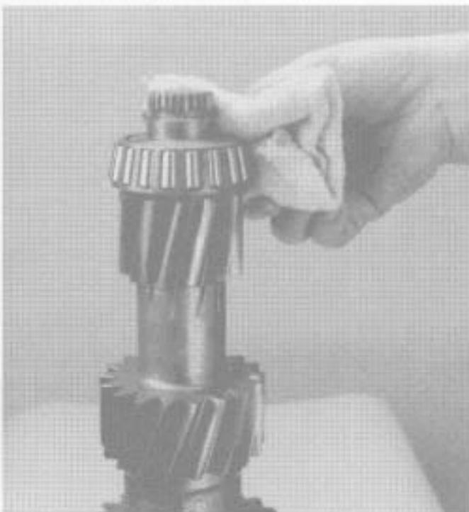
5. Heat and install the rear countershaft bearing.
