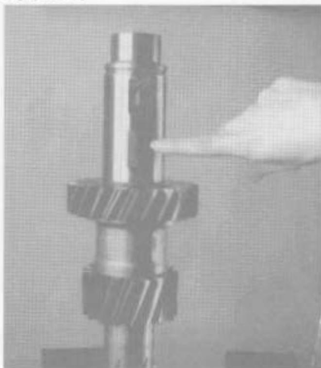
13. Remove 4th gear key from the countershaft
