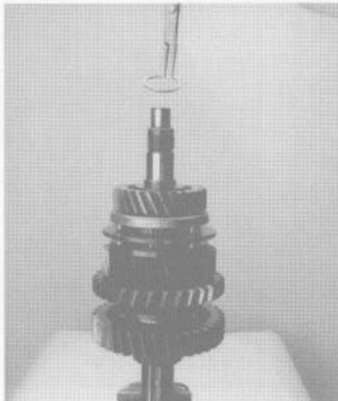
9. Remove 3rd speed gear retaining snap ring.
