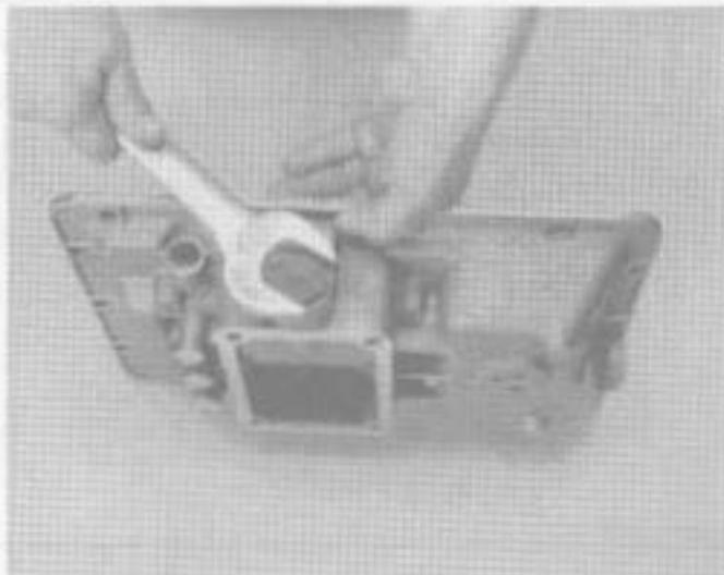
3. Install the reverse plunger gasket and plug. Tighten the reverse plunger plug to the recommended torque.
