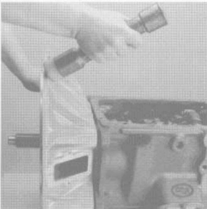
2. Jar clutch housing with a rubber mallet and pull from the transmission case.
