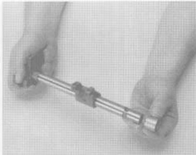
7. If necessary, remove the front spacer from 1st-reverse shift bar.
