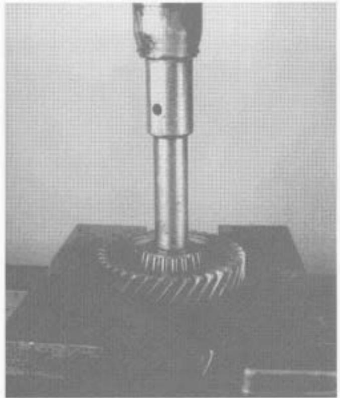
10. Use the countershaft drive gear rear face as a base, then press the drive gear, snap ring, and bearing from the countershaft.
