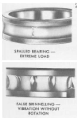
2. Lubricate bearings which are not spalled or pitted and check for axial and radial clearances. Replace bearings with excessive clearances.
