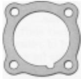
1. **GASKETS** - Use new gaskets throughout the transmission as it is being rebuilt. Make sure all gaskets are installed, as omission of gasket can result in oil leakage or misalignment of bearing covers
