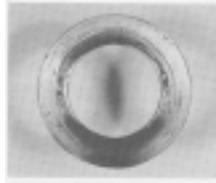
1. Check surfaces of all thrust washers. Washers scored or reduced in thickness should be replaced.
