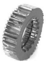
Replace lube and bearings when damage to gearing appears similar to or worse than damage on this gear. Replacement is required due to fine particle contamination.
