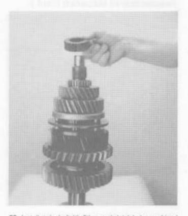
Install mainshaft 4th-5th speed clutch hub, machined surface facing up.
