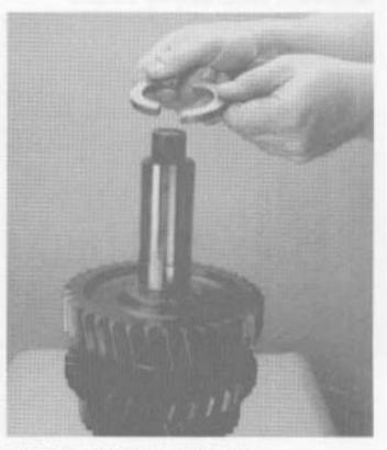
17. Remove the 1st gear split washer.
