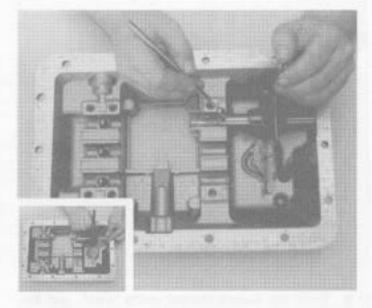
Position 1st-reverse yoke assembly in the shift bar housing (inset). Install the 1st-reverse lock pin in the yoke assembly.
