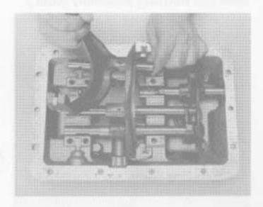
Position the 4th-5th yoke assembly in the housing assembly as shown.
