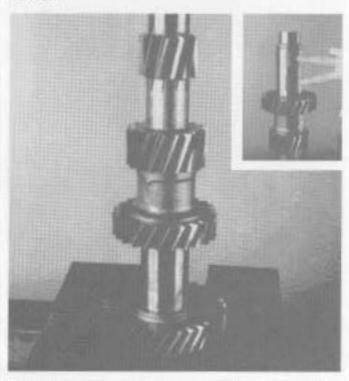
Install 4th and 5th speed gear keys in the countershaft keyways (inset). Align 4th speed countershaft gear keyway to shaft key. Press 4th gear on the countershaft, long hub to shaft front.
