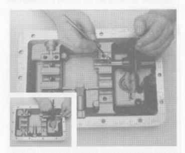
Remove the 1st-reverse lock pin from the 1st-reverse shift yoke assembly. Remove the 1st-reverse shift yoke (inset).
