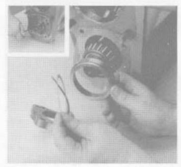
Remove the two set screws (inset). Remove the bearing retainer, outer race, and shims.
