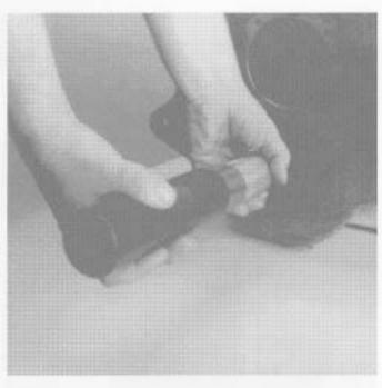
If previously removed, install the snap ring, countershaft front bearing race (from inside of case) and front case bore plug. Coat the outer diameter of bore plug with Loctite #510 before installing.
