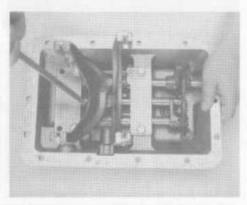
Lay the shift bar housing on the work bench. Remove two capscrews as shown and shift 4th-5th yoke assembly into 4th speed position with a screwdriver.
