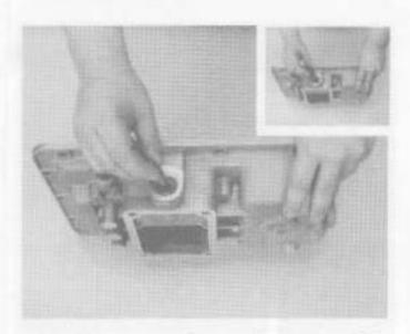
Install the reverse plunger spring (inset), and the reverse plunger stop.
