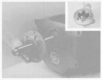
Remove the four capscrews from the front bearing cover and remove the cover and shims. The front bearing cover shims can come off with the front bearing cover. If necessary, remove the oil seal from the cover (inset).
