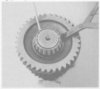
Use a screwdriver and snap ring pilers to move the snap ring out of snap ring groove and against the bearing back.
