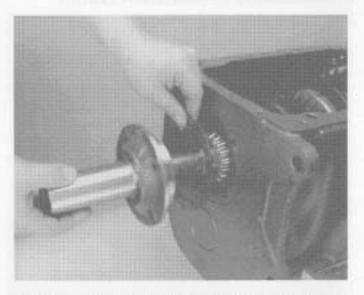
31. Install input shaft bearing cover, gasket, and capscrews. The front bearing cover lubrication oil groove must be at the top. Apply Loctite #262 to threads of capscsrews and tighten to recommended torque.
