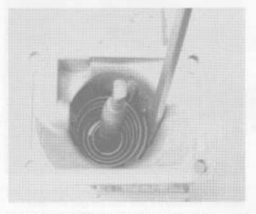
Remove the shift lever grip and boot from the shift lever, secure assmbly in a vise with the housing bottom up. Use a large screwdriver to twist between spring and housing, forcing the spring from under the housing lugs. Do one coil at a time.
