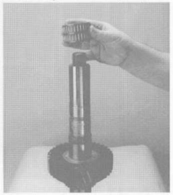
5. Install mainshaft reverse gear bearing.
