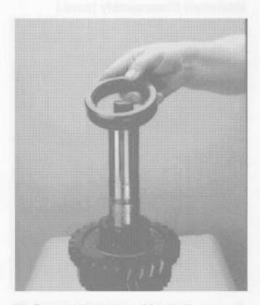
21. Remove the 1st-reverse sliding clutch.
