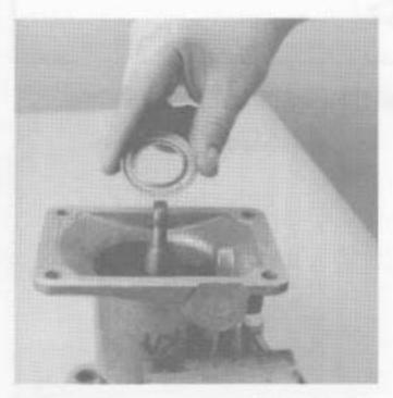
Remove the washer and gearshift lever from the housing. Remove the boot from the gear shift lever.
