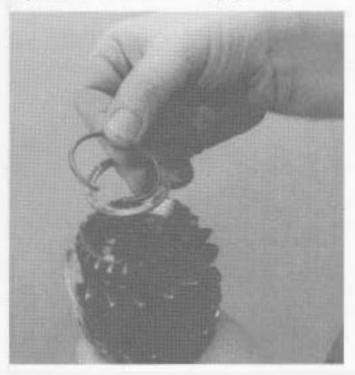
If necessary, remove the retention snap ring and the bearing retention ring.
