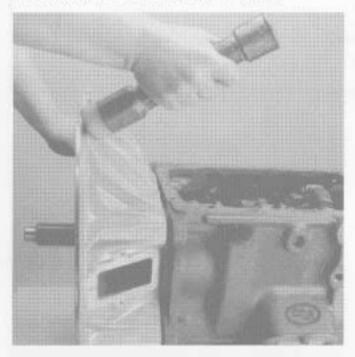
Jar clutch housing with a rubber mallet and pull from the transmission case.
