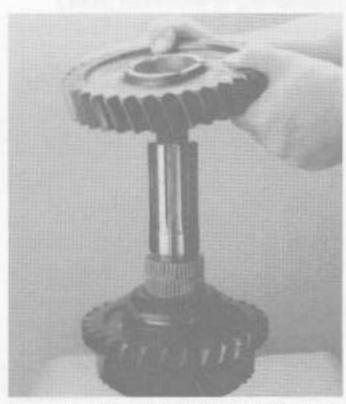
Install mainshaft 1st gear over the two rows of needle bearings, with clutching teeth down. Be careful not to catch the needle roller bearings.
