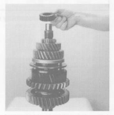
6. Remove 4th-5th speed clutch hub.
