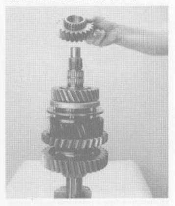
7. Remove the 4th speed gear.
