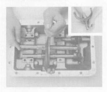
Install the 2nd-3rd yoke assembly interlock pin (inset).
