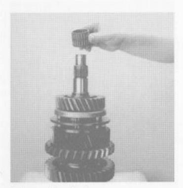
8. Remove 4th gear bearing.
