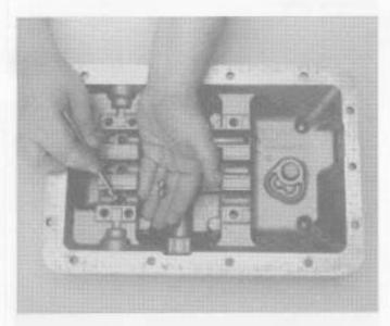
Remove the four interlock balls, the three detent balls, the three back up light switch balls, and the three springs from the shift bar housing.
