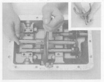
Remove 2nd-3rd yoke assembly and interlock pin (inset).
