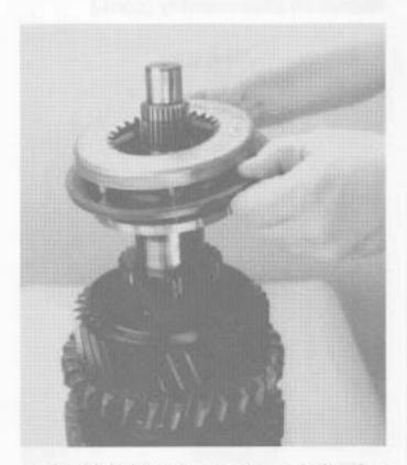
Remove the 3rd gear synchronizer cup and synchronizer assembly.
