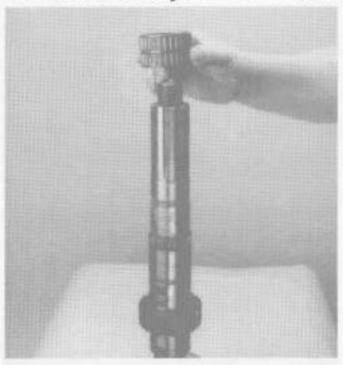
Install the mainshaft in a vise equipped with wood or brass jaws, mainshaft rear facing up. Lubricate and install mainshaft 2nd speed gear bearing.
