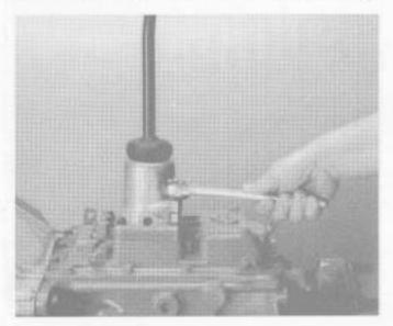
Turn out four capscrews and remove the tower assembly and gasket from the shift bar housing.
