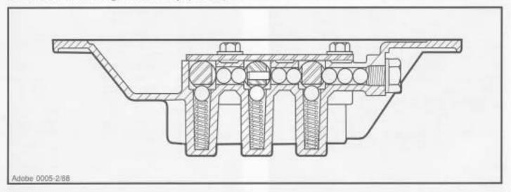
Install interlock balls, detent balls and springs in the following sequence; position (3) balls in the reverse light switch bore and install 1st-reverse detent spring and ball.
