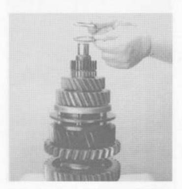
Install thrust bearing and bearing race on the mainshaft 4th-5th clutch hub.
