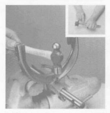
If shift blocks or shift yokes were removed, align shift yoke or block with alignment hole in the shift bar and insert lock pin.
