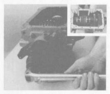
Lock the transmission by engaging two mainshaft gears as shown (inset). Use a large breaker bar to turn the retaining nut from the output shaft.
