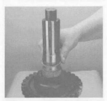
10. Coat the mainshaft 1st gear position with a high quality grease. Lay a row of needle bearings around the mainshaft, 44 needle bearins. Place a spacer ring over the top of the bearings. Lay a second row of 44 needle bearings around the mainshaft on top of the spacer ring. Install a spacer ring over the top of the second row of needle bearings.
