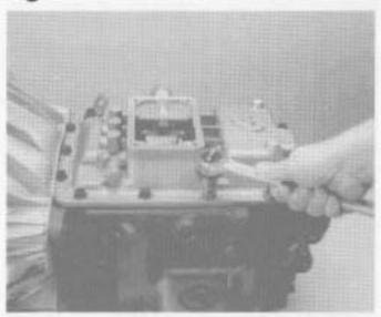
Install the remaining capscrews and fighten to the recommended torque.
