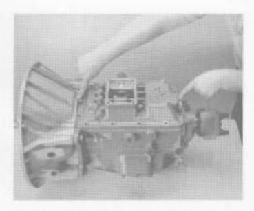
Apply Loctite #262 to threads of capscrews. Install two capscrews into shift bar housing alignment holes and tighten to the recommended torque.
