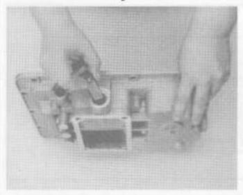
Place the shift bar housing on its side as shown and install the reverse plunger.
