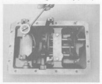
Install the remaining two capscrews and tighten capscrews to recommended torque.
