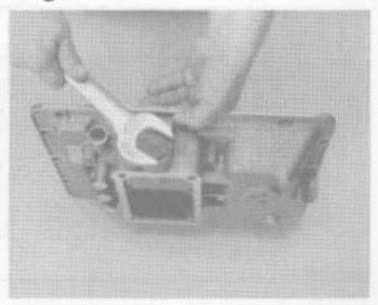
Install the reverse plunger gasket and plug. Tighten the reverse plunger plug to the recommended torque.
