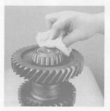
Heat and install the front countershaft bearing.
