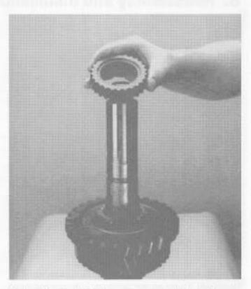
7. Install mainshaft 1st-reverse speed clutch hub.
