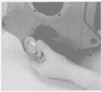
If the countershaft front bearing race is to be replaced, drive the bore plug through the front of the transmissison and drive the race to the rear toward the case's inside.
