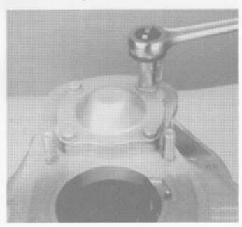
Install the countershaft rear bearing cover and gasket.
