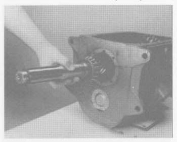
Install the input shaft by aligning clutching teeth on drive gear with teeth in mainshaft 5th speed synchronizer cup.
