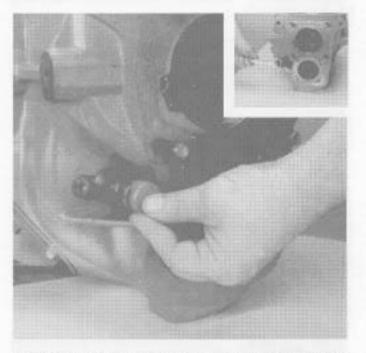
8. Insert the reverse idler shaft through the case and idler gear needle bearings. Install the reverse idler retainer and capscrew (inset). Make sure the idler shaft locking groove lines up with the capscrew hole. Tighten the capscrew to the recommended torque.
