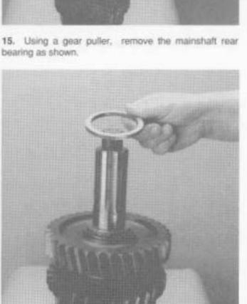
Remove the 1st gear split washer retaining ring.
