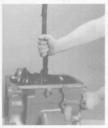
Wrap a sling or rope around the 2nd-3rd synchronizer. Use a hoist to remove the mainshaft assembly from the transmission case.
