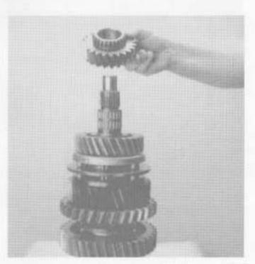
Install mainshaft 4th speed gear, clutching teeth facing up.
