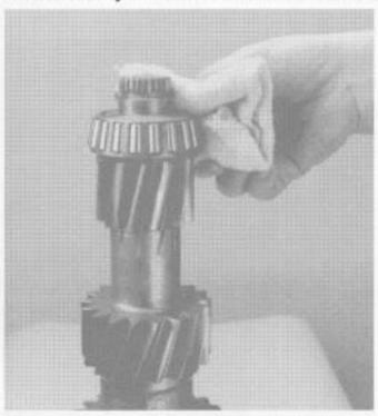
Heat and install the rear countershaft bearing.
