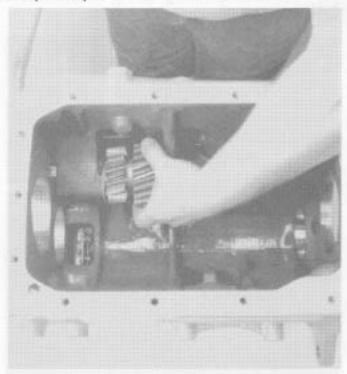
Use grease on the two reverse idler thrust washers to hold in place. Install reverse idler gear with tangs of washers in housing groove, with the small reverse idler gear to the rear.
