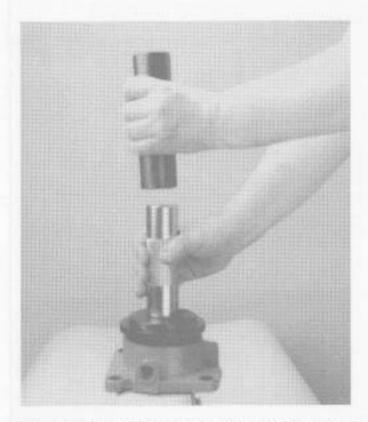
If a new oil seal is required, install using a flanged driver. Coat the oil seal outer diameter with Loctite #510.
