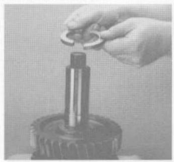
Install a locating ball on the mainshaft. Install 1st speed gear split washer, so the split rings join at the locating ball.
