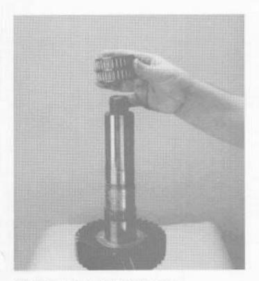
24. Remove the reverse gear bearing.
