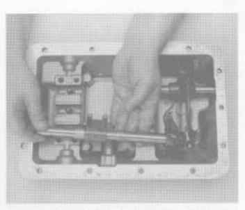
Remove 1st-reverse bar assembly. If necessary remove the front spacer from 1st-reverse shift bar (inset).
