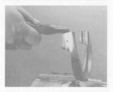
If the yoke pads are to be replaced, remove worn pad from shift yoke, install new pad and bend tabs over top and bottom of yoke.
