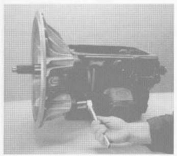
1. Remove the four retaining bolts as shown.
