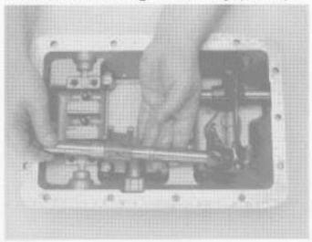
Position 1st-reverse bar assembly in the housing assembly as shown.
