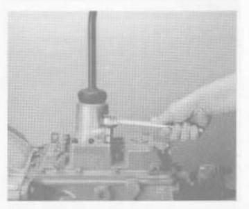
Coat the retaining capscrews threads withLoctite #262 and install. Tighten the capscrews to the recommended torque.
