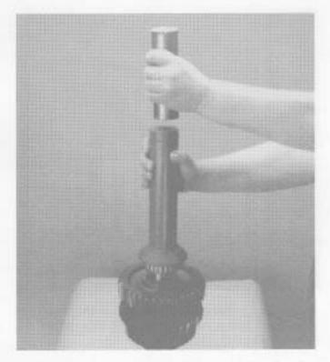
Using a bearing driver, install mainshaft rear bearing as shown.
