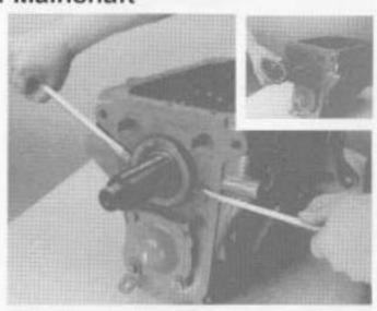
Remove speedometer drive gear (inset). Tap on the front of the main shaft to move the mainshaft rearward about 1/4". Use pry bars to remove the rear bearing cup and locating snap ring.
