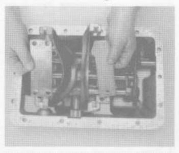
Remove the rest of the capscrews and the two retainers.
