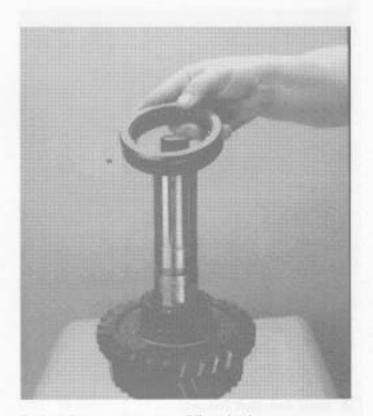
8. Install 1st-reverse gear sliding clutch.
