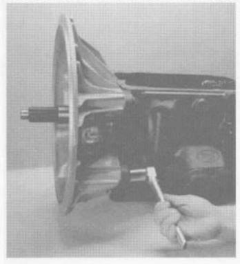
Position the transmission as shown. Place the clutch housing on the transmission case. Install the four retaining bolts and tighten to the recommended torque.
