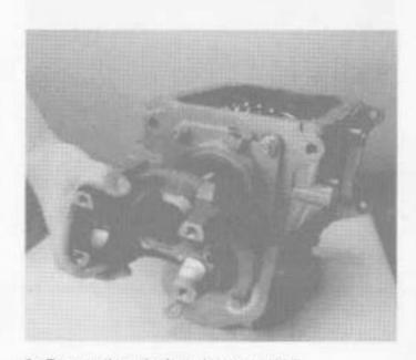
2. Remove the yoke from the output shaft.
