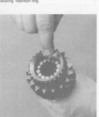
If necessary, remove the 14 roller bearings from the main drive gear bearing pocket.
