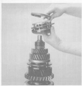
Install the mainshaft assembly in a vise equipped with soft jaws or wood, shaft front facing up. Remove the 4th-5th speed synchronizer and cups.
