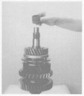
21. Install mainshaft 4th gear bearing.
