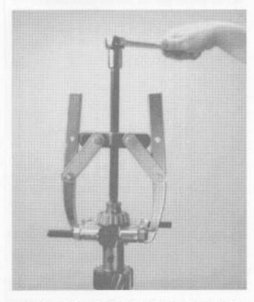
Position gear puller and clamp behind the rear countershaft bearing and remove the bearing.
