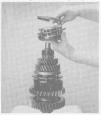
Install 4th-5th speed synchronizer and cups over the mainshaft 4th-5th clutch hub.
