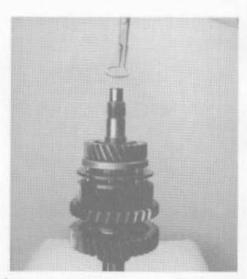
Install mainshaft 3rd speed gear retaining snap ring in the snap ring groove.
