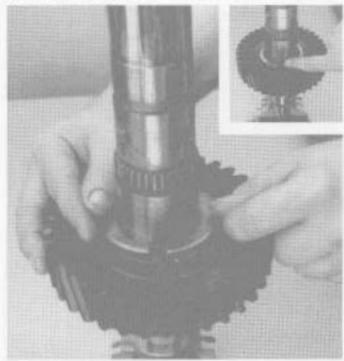
Install locating ball (inset) and 2nd gear split washer so the split rings join at the locating ball.
