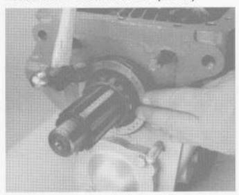
Install the main shaft rear outer bearing race in the output shaft bearing bore.
