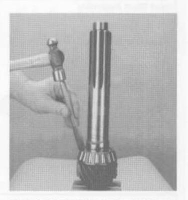
Use a chisel to remove the bearing cage and rollers. Install bearing puller and remove the bearing race from the input shaft.
