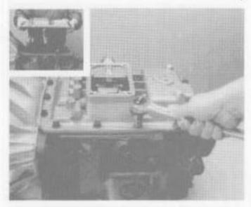
Shift the transmission into neutral position, remove the capscrews, and lift the shift bar housing and gasket from the case (inset).
