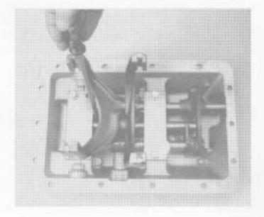
Place the shift yokes in neutral and install the two retainers and the four capscrews as shown. Tighten the capscrews to the recommended torque. Shift 4th-5th yoke assembly into 4th speed position.
