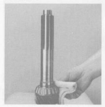
Heat the input shaft bearing and install the bearing on the input shaft.
