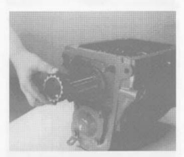
32. Install the speedometer drive gear or rotor on the output shaft.
