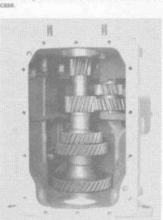
10. Position the transmission case on end as shown. Position the countershaft assembly into the front bearing race.
