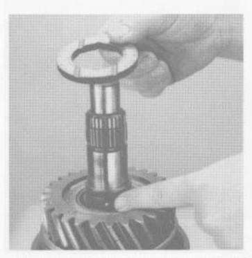
Remove 3rd speed gear thrust washer. Remove the locating ball.
