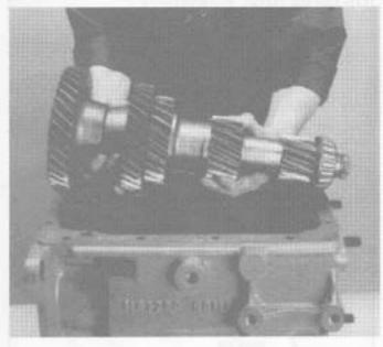
Move the countershaft assembly to the rear and lift it from the transmission case.
