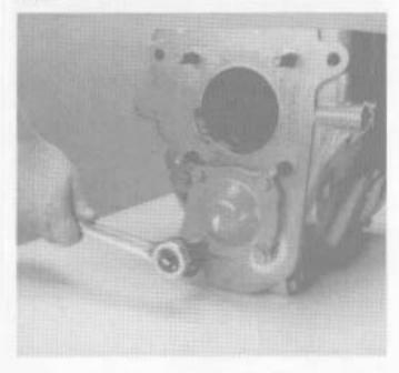
Remove the four capscrews and the countershaft rear bearing cover and gasket.
