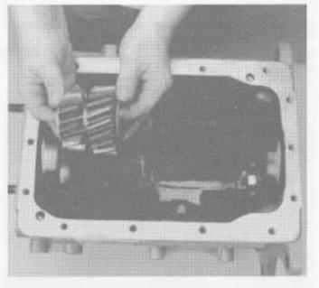
Remove the reverse idler bearings, spacer, and thrust washers.
