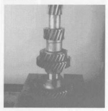
Press 5th speed countershaft gear on, long hub to shaft rear.
