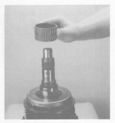
12. Remove the 3rd gear bearing.
