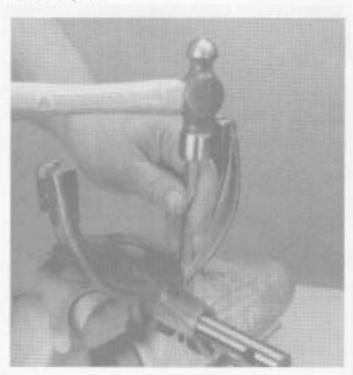
If necessary, shift blocks and shift yokes can be removed by driving lockpin from shift bar with a punch and hammer as shown.
