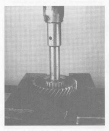
Use the countershaft drive gear rear face as a base, then press the drive gear, snap ring, and bearing from the countershaft.
