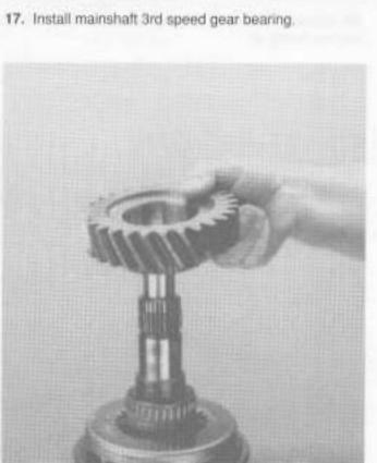
Install mainshaft 3rd speed gear, clutching teeth facing down.
