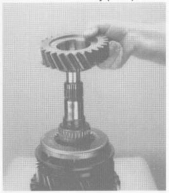
11. Remove the 3rd speed gear.
