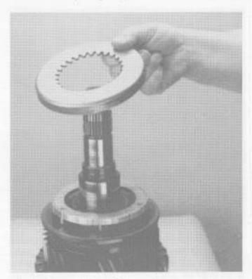
Install the mainshaft 3rd speed gear synchronizer cup as shown.
