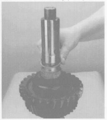
19. Remove the bearing rollers and spacers.
