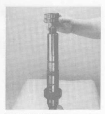
28. Remove 2nd gear bearing.
