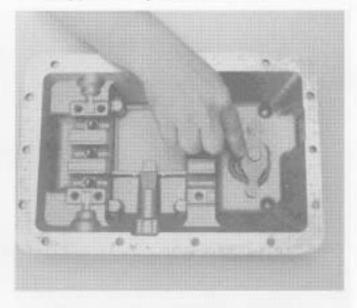
Seat the 1st-reverse actuator in the shift bar housing, over the actuator pivot pin, as shown.
