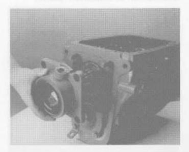
35. Coat both sides of a new rear bearing cover gasket with Loctite #510, and position the gasket on the rear bearing cover. Install the rear bearing cover, position the lubrication oil groove with case hole.
