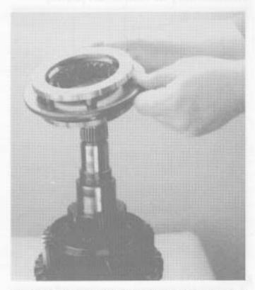
Reposition mainshaft in vise so front is up. Install the mainshaft 3rd speed gear synchronizer assembly.
