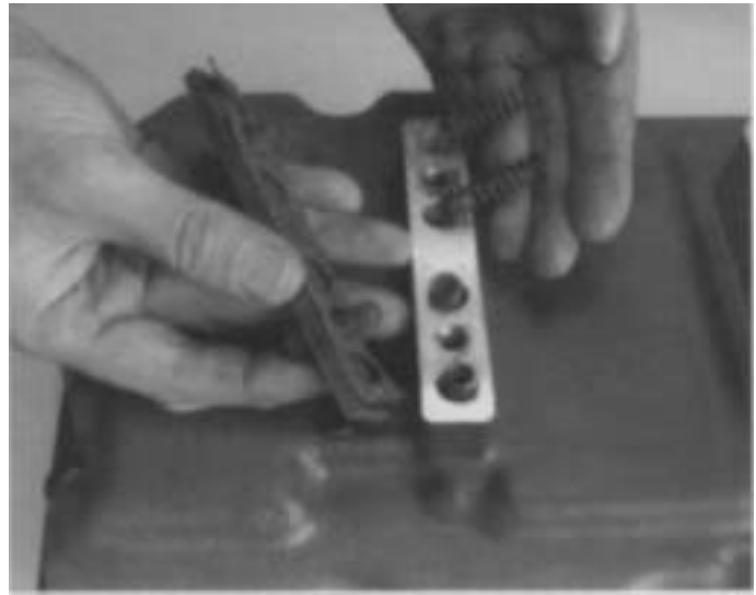
17. Install the four detent springs, gasket and detent spring cover on the shift bar housing.
