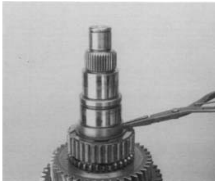
12. Install the 3rd-4th speed shift hub retaining snap ring in the mainshaft snap ring groove.
