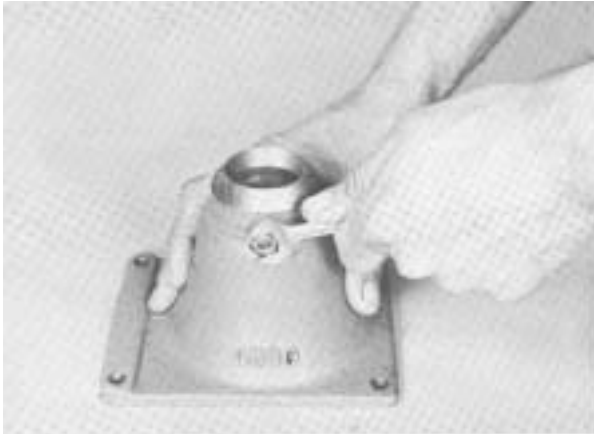
1. Install lockwasher and nut on gear shift lever pivot pin.
