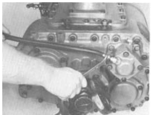
6. Remove air lines from range shift cylinder.
