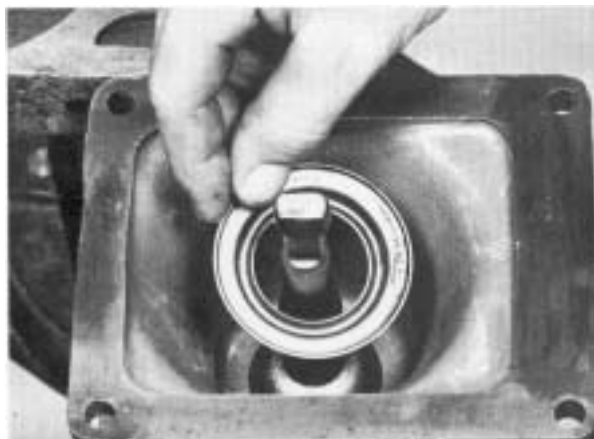
3. Place the tension spring washer in housing.
