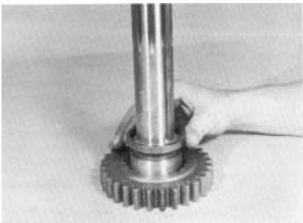
3. Install spacer on shaft.
