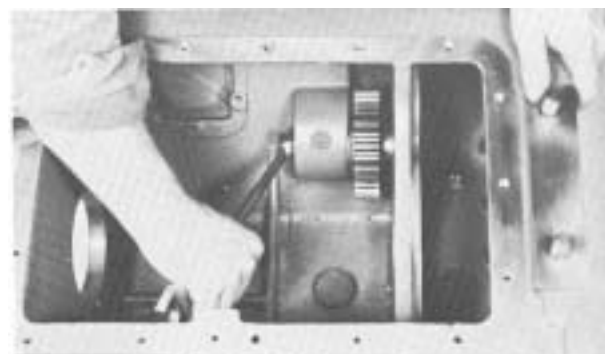
6. Install elastic stop nut and retainer washer on shaft. (if desired the auxiliary countershaft front bearing can now be installed in the right reverse idler bore).
