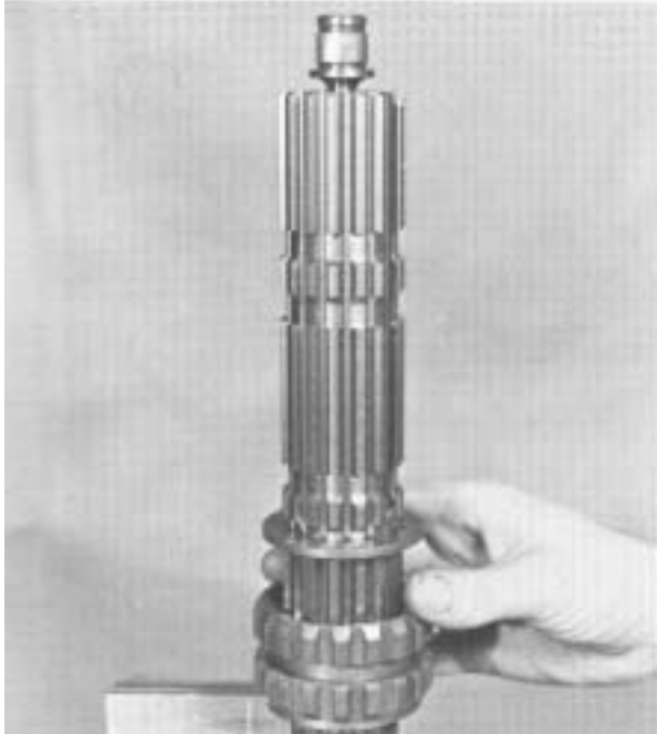
4. Install the first speed gear washer, flat side up, engaging keyway with key. (use 14274 low limit washer).
