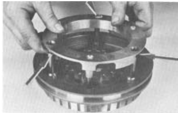
2. pull direct synchronizer from blocker pins of low speed synchronizer. Place cloth over ring during removal as springs direct ring will be released at arrow locations.
