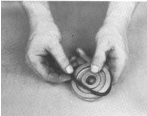
8. Install O-ring on OD of piston.
