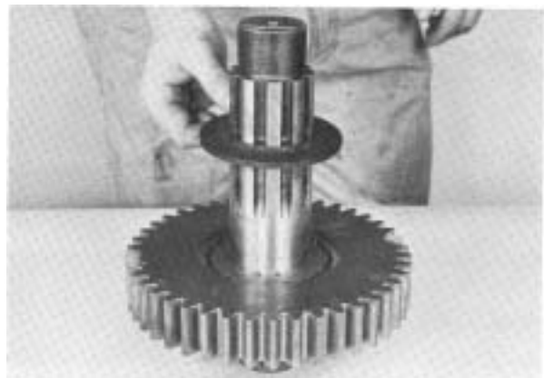
5. Install rear washer on shaft.
