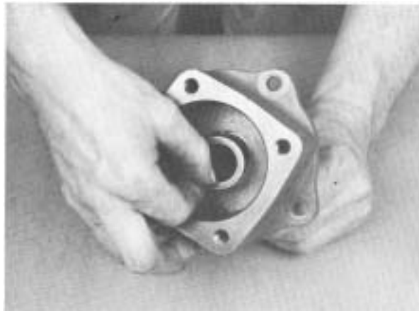
2. Install washer in shift cylinder against O-ring.
