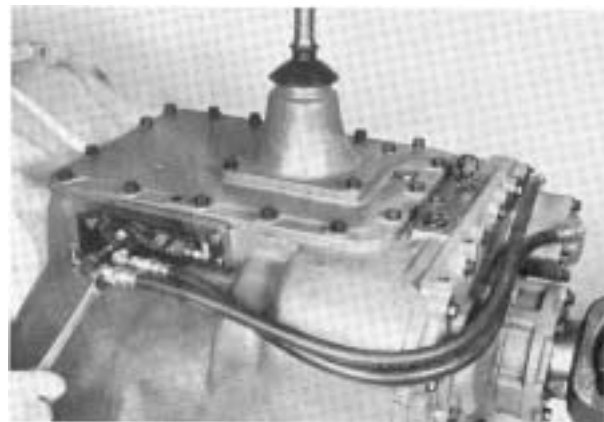
7. Install the Low range air line between port in range cylinder and front port to air valve.
