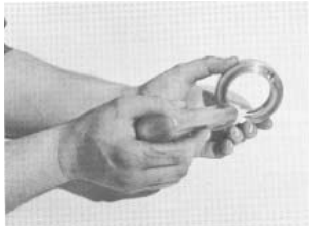
5. Apply grade AVV loctite sealant to threads of drive gear nut. Also apply sealant to threads of shaft.
