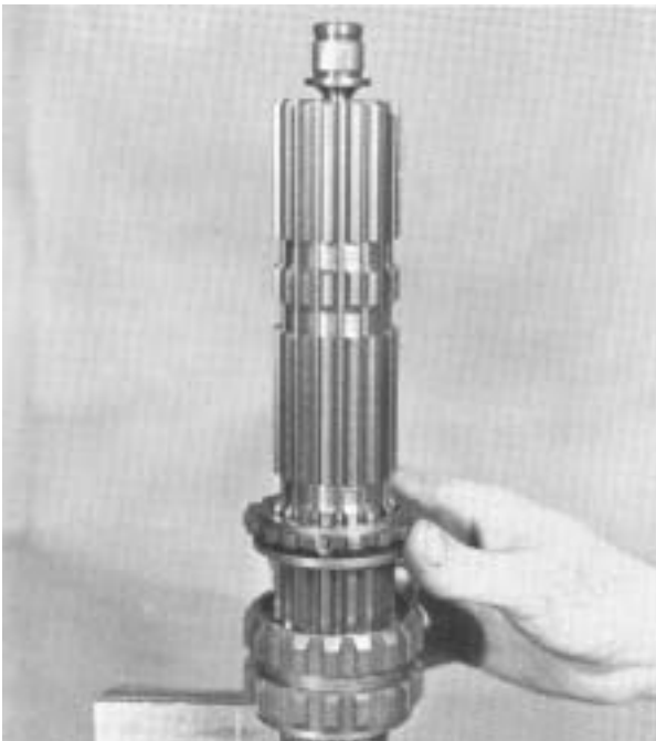
5. Install the first speed gear spacer, flat side next to washer.
