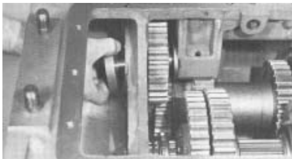
4. Place thrust washer and gear into position in case and insert shaft through gear and into boss.
