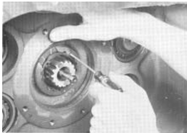
with reverse idler gears and install snap ring in ID of gear.
