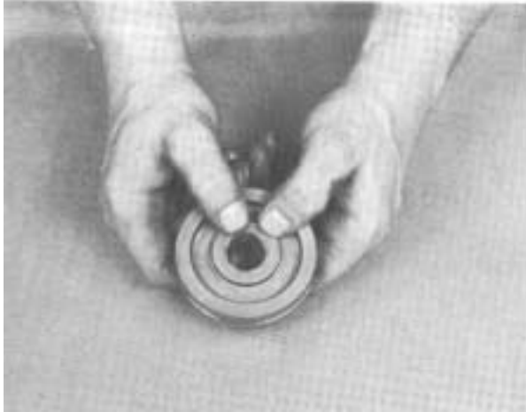
7. Install O-ring in ID of piston.
