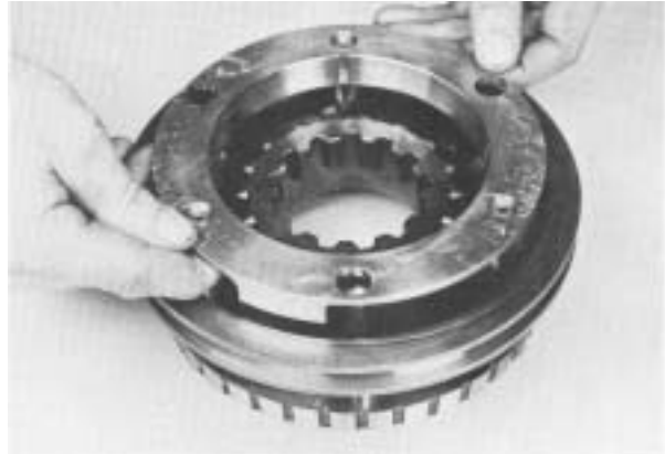
3. Place direct synchronizer over pins of the low speed synchronizer with springs against the low speed blocker pins.
