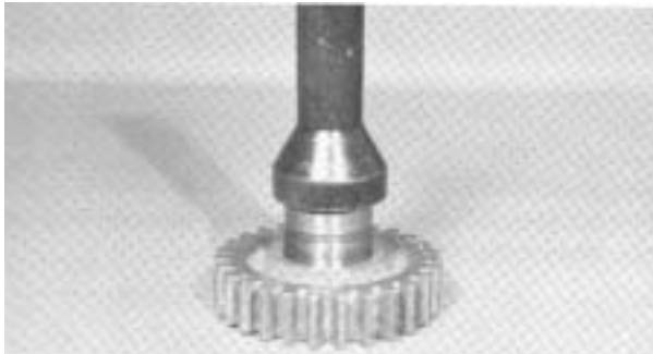
3. press needle bearing into bore of reverse idler gear.
