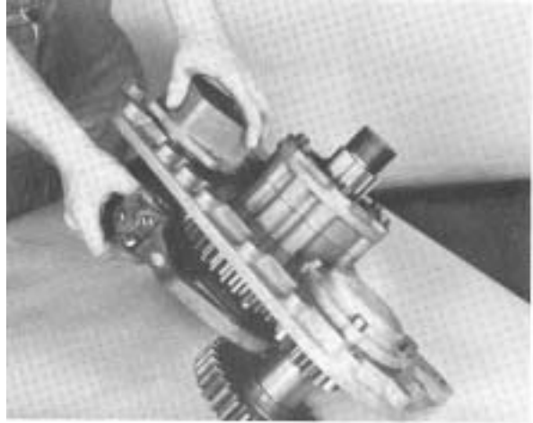
6. Remove the shifting yoke and shift cylinder
