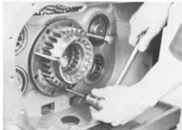
5. Remove lockwire and capscrews, insert puller screws and pull the auxiliary drive gear assembly from case bore.
