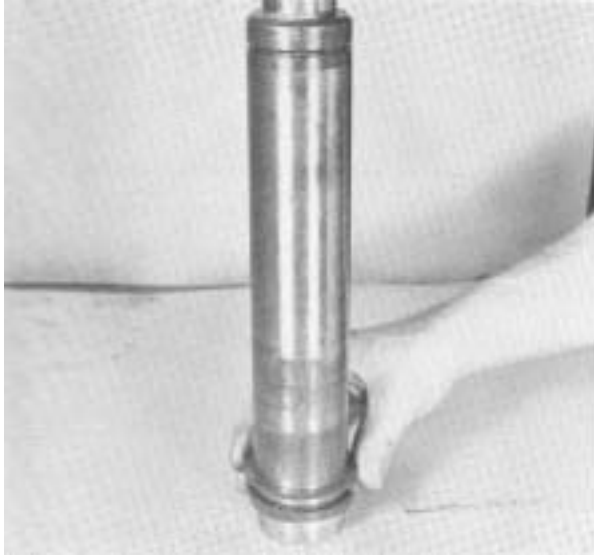
1. Install the countershaft front spacer.
