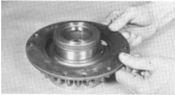
1. Place retainer ring on auxiliary drive gear.
