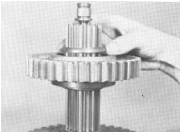
13. Install the 2nd speed gear washer in hub of gear, flat side down.
