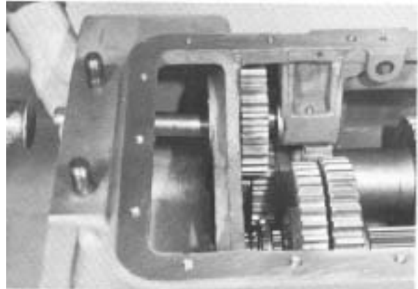
5. seat shaft in bore; make sure needle bearing is aligned with bearing sleeve.
