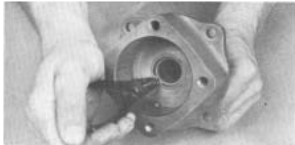
7. Remove snap ring from bore in shift cylinder; this will free washer and O-ring installed under snap ring
