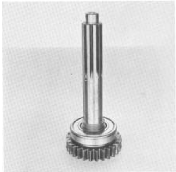
4. Drive gear bearing installed on shaft; a press fit.
