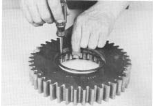
3. Install snap ring in ID of low speed gear.
