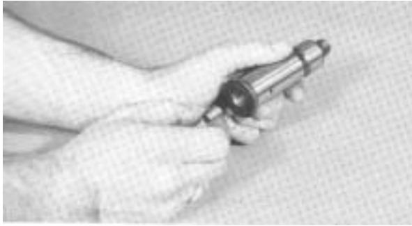
1. Install plug in reverse Idler gear
