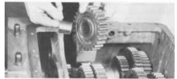
6. Remove bearing inner sleeve from gear; press bearing inner race from gear if necessary.
