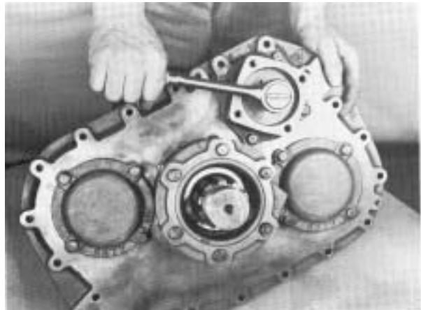
2. Turn nut from air cylinder shifting bar
