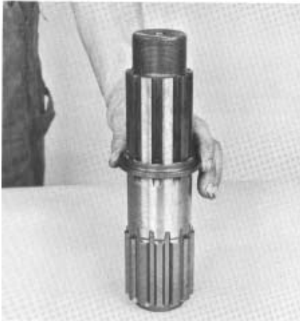
1. Install stepped washer on auxiliary mainshaft.
