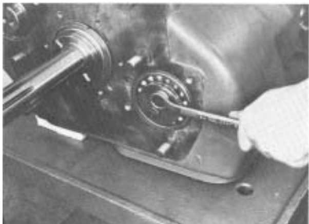
6. Install the bearing retainer plate on front of left countershaft. Tighten and wire securely.
