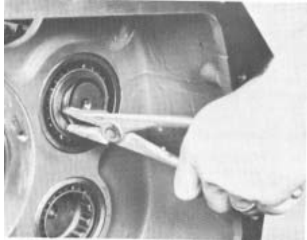
10. Install the snap ring on rear of right countershaft.
