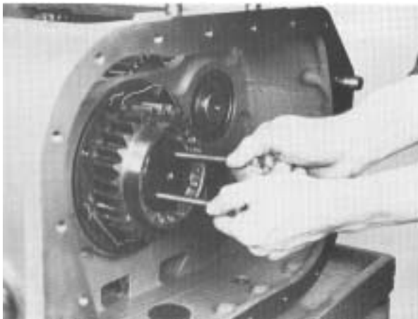
2. Insert puller screws and remove quill support plate from gear.
