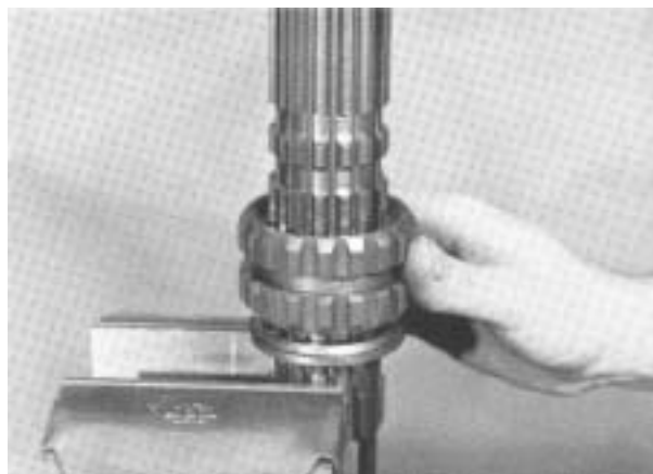
3. Install the first-reverse sliding clutch on shaft.
