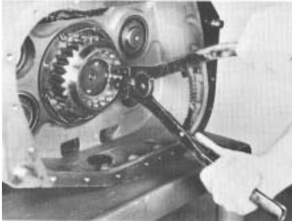
1. Remove large snap ring from ID of auxiliary drive gear.
