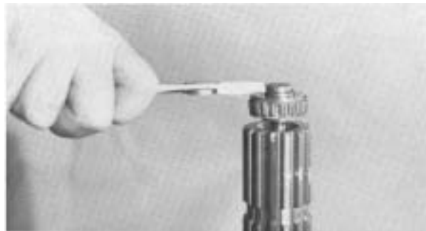
6. Place mainshaft in vise and remove snap ring from front quill.
