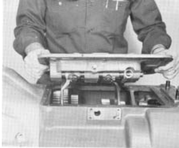
7. Install the shifting bar housing on transmission, fitting yoke forks into slots in sliding clutch gears.
