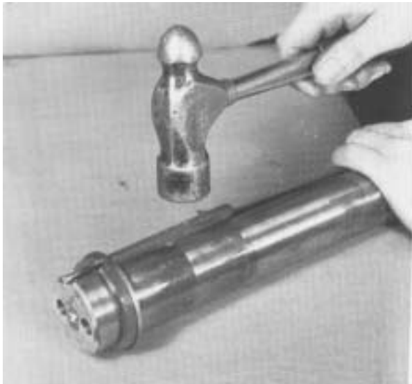
2. Install the front key in countershaft.
