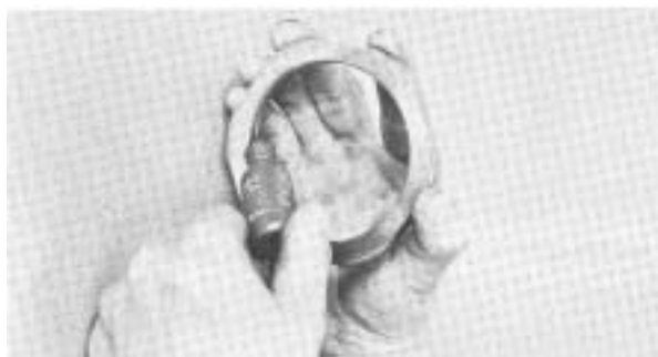
3. Apply loctite Grade AVV sealant to threads of auxiliary drive gear nut and drive gear.
