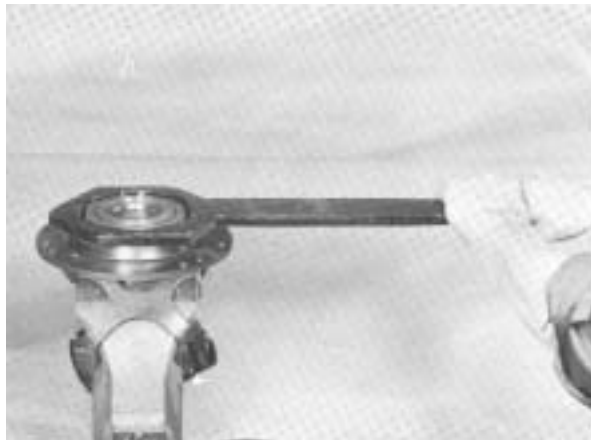
6. Remove auxiliary drive gear bearing nut, left-hand thread. Press retainer ring and bearing from drive gear.
