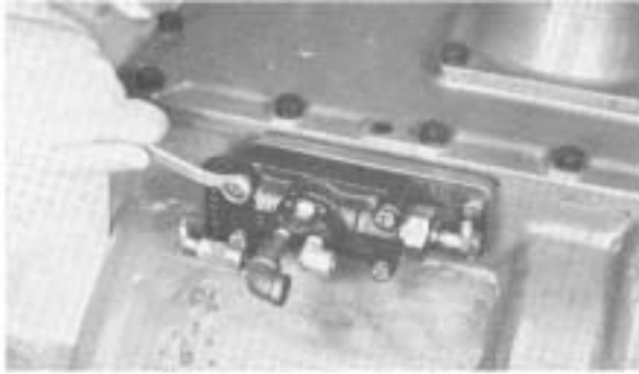
7. remove the air shift valve.
