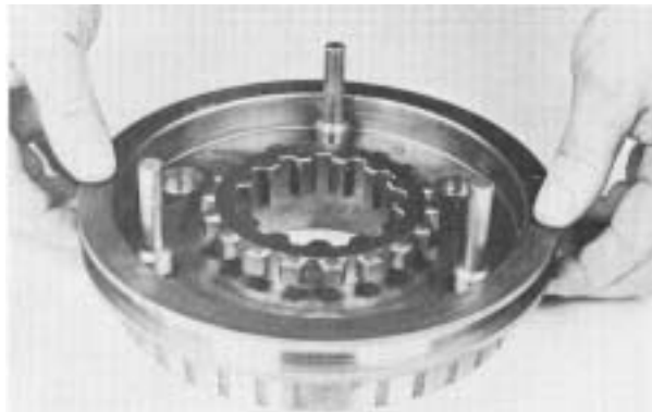
3. Remove sliding clutch gear from low speed synchronizer.
