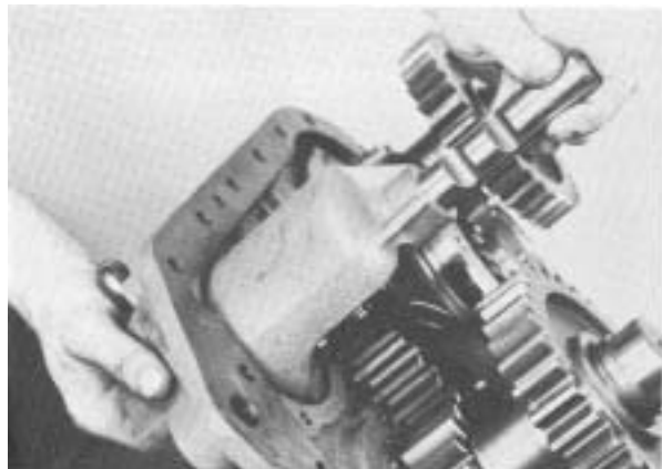
5. Install the shifting bar; align notches with cap screw bores in yoke.
