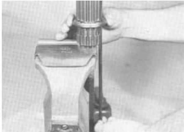
2. Install the reverse gear washer on shaft, flat side down, and insert key through keyway in washer. (use 14274 low limit washer).
