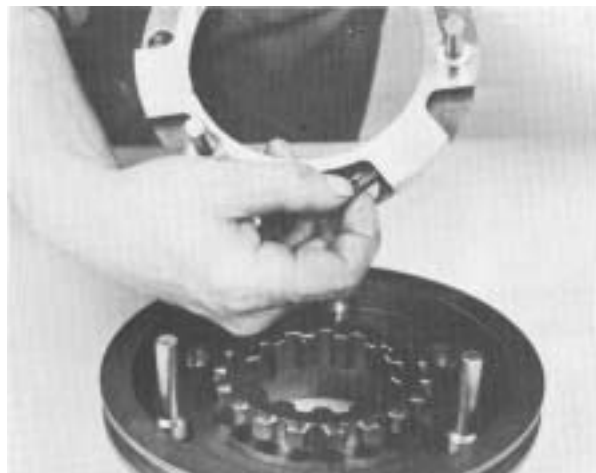
2. Install the three springs in direct synchronizer.
