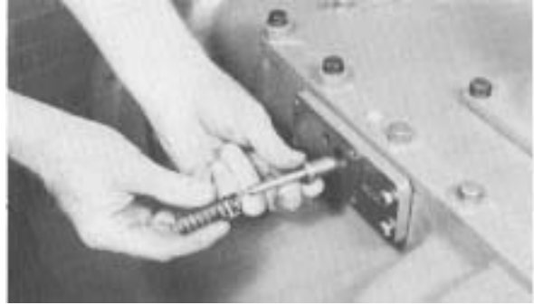
9. Remove spring and actuating pin.
