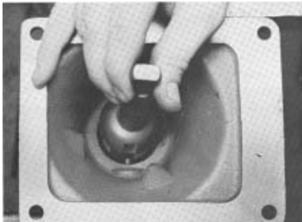
2. Install gear shift lever in housing, inserting pivot pin in slot in pivot ball of lever.
