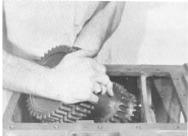
12. Place the right countershaft assembly (45-Tooth PTO gear) into position in case. Do not install bearings.
