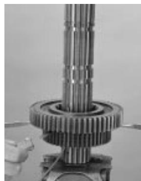
11. With the missing internal splines aligned with the plastic line, install a sliding clutch.
