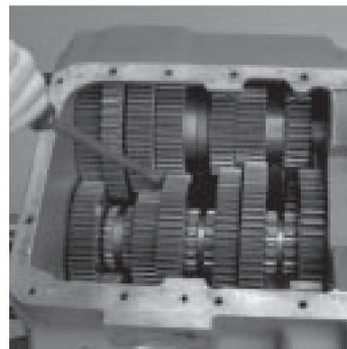
5. Use a rolling head prybar (crow's foot) to work the mainshaft rear bearing from its bore.
