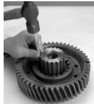
6. If necessary, remove the bushings from inside the coupler.
