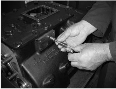
3. Remove interlock parts (pin, spring, and sleeve).
