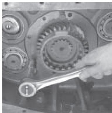
4. If it does not move easily, it may be necessary to install three cap screws in the threaded holes on the retainer plate. Tighten the three screws evenly to force the auxiliary drive gear assembly from the case. The three threaded holes are only found on earlier models.
