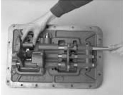
15. Holding the top bar notched-end, start installation. As the bar passes the rear boss, position the shift block.
