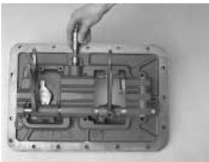
6. Remove the actuating plunger from the center top bore boss.
