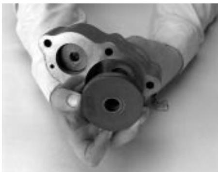
8. Remove the range and reduction pistons from the cylinder bores.
