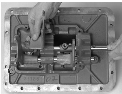
5. From the middle yoke bar, remove the shift yoke and shift block. As the neutral notch in the bar clears the rear boss, remove the small interlock pin from the notch bore.
