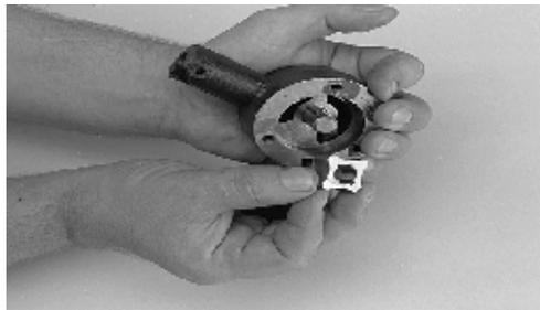
7. From the drive shaft keyways, remove the two (2) keys.
