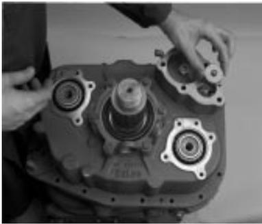
6. Install deep reduction piston with flat side to rear. Install nut and torque to 50-65 Lb•ft.
