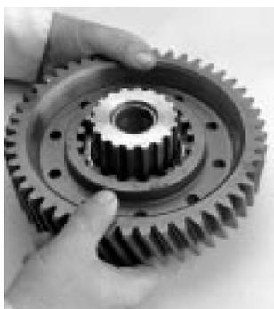
5. Assemble gear over coupler.
