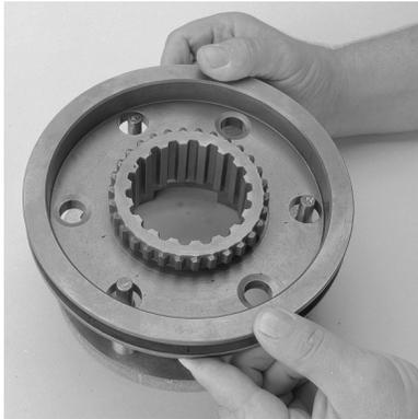
1. On the bench place the larger LO range synchronizer ring face down with pins up.
