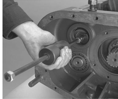
5. As the idler shaft and idler plate are removed, remove the thrust washers and gear.
