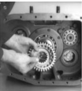
4. Slide the auxiliary driver gear over the mainshaft splines. Install the rear snap ring in the mainshaft groove.
