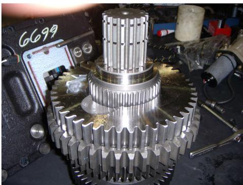
20. Install the clutch hub with the bezel facing up.
