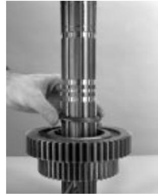
9. Push the air line up to lock the washers on the mainshaft.
