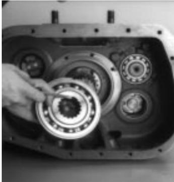
1. Press the inner sleeve into the rear mainshaft bearing.
