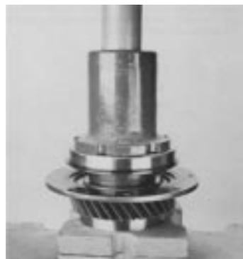
3. Install the snap ring in gear hub groove to retain the bearing.
