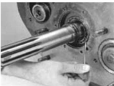
7. Remove the drive gear internal snap ring.
