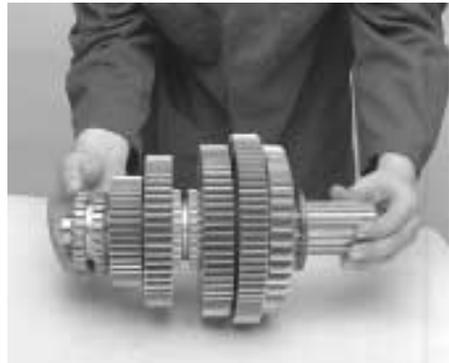
2. Place the mainshaft in a vertical position, pilot end down. Remove the reverse gear, clutch hub, and sliding clutch.
