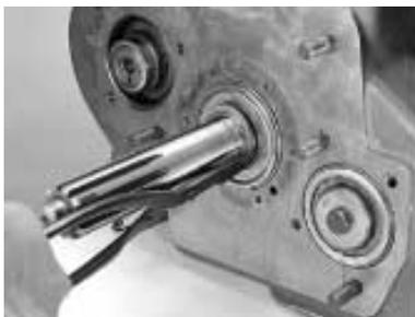
3. From the input shaft groove, remove the bearing retaining snap ring.
