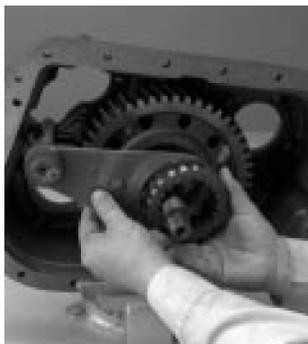
8. Remove the sliding clutch and the reduction yoke assembly from the auxiliary housing.
