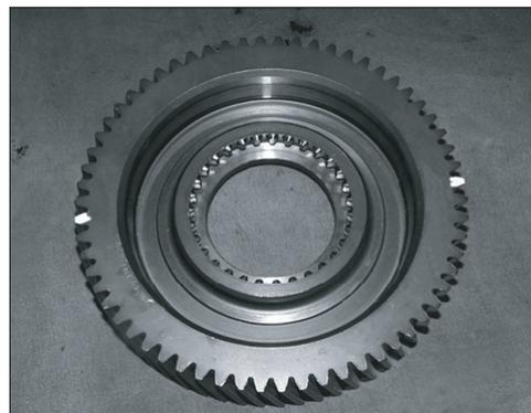
3. Locate the two stamped "O's" on the Countershaft Reduction gears and mark both teeth with a highly visible paint, preferably a yellow or white.
