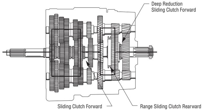
Figure 2-9. Low Range Selected (Range Sliding Clutch Rearward)
