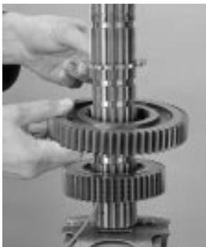
6. With clutching teeth down and engaged with the spacer external splines, position the proper gear on the mainshaft. If necessary, refer to the illustrated parts list to determine gear order.
