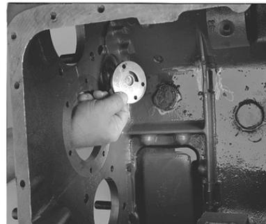
7. If necessary, the front case plug can be removed from the case. To remove, insert a bar from inside the case and tap the plug out.
