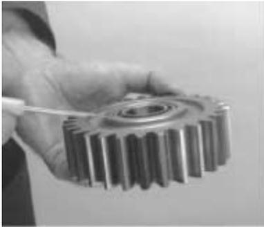
2. Position the gear in the case. The gear's long hub is positioned forward.
