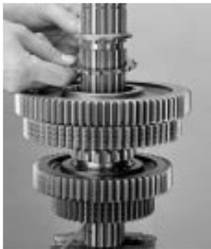
17. Position another spacer against the previously positioned gear, engaging the spacer external splines with gear clutching teeth.
