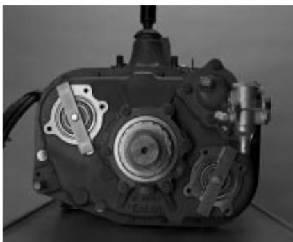
3. Install countershaft retaining strap.
