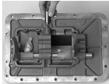
10. Holding the middle bar notched-end, start installation. As the bar passes the rear boss, position the shift block.
