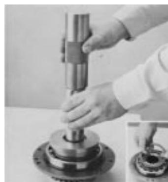
5. Install the auxiliary drive gear assembly on the mainshaft rear. Use a flanged-end driver to fully seat the assembly in the case bore.
