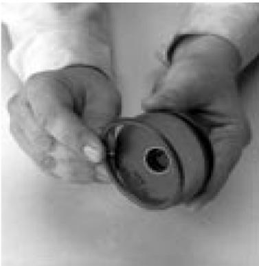
9. If necessary, remove the O-rings from the range cylinder bore and the reduction cylinder bore.
