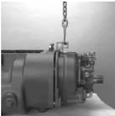
6. Attach an auxiliary section hanger bracket to the auxiliary section top.
