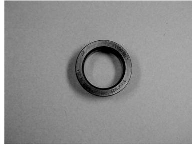
5. Temporarily install a spare countershaft inner race inside the front roller bearing for installation.
