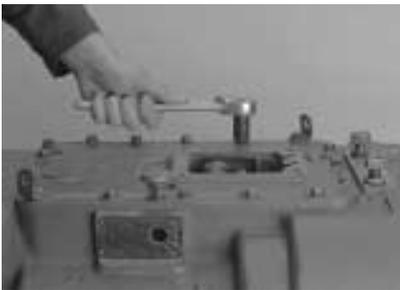
4. From the shift bar housing rim, remove the retaining cap-screws.
