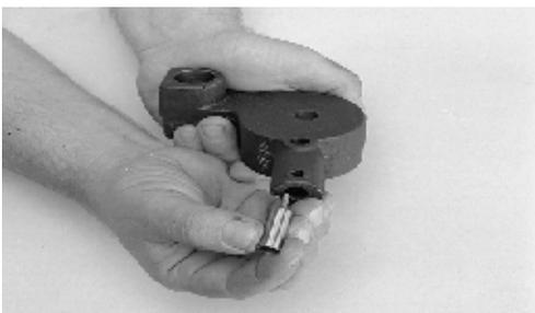
12. From the housing bore, remove the relief valve.
