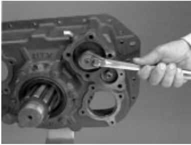
5. Install range piston with flat side to rear. Install range piston nut and torque to 70-85 Lb•ft.
