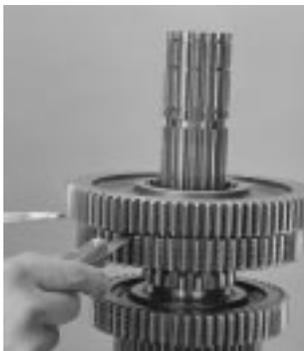
20. Insert two large screwdrivers between the two gears. Apply slight downward pressure to spread the gears evenly. Between the gear hub and mainshaft spacer, insert 0.006" feeler gauge and 0.015" feeler gauge. If out of tolerance, change the washer against the mainshaft spacer. Refer to information before stepped procedures for further information.
