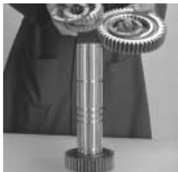
6. Remove the offset washer and sliding clutch, and then remove the offset washer and 3rd gear.
