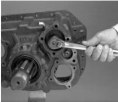
5. Install range piston with flat side to rear. Install range piston nut and torque to 70-85 Lb•ft.
