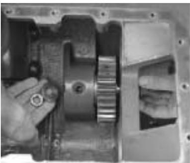
7. Install the flat washer over the shaft threaded portion.
