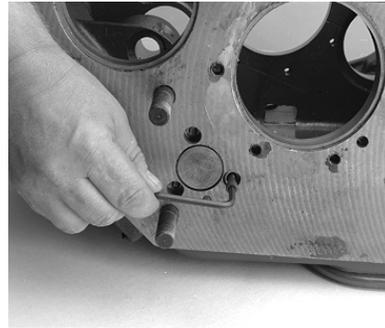
8. Bend the suction tube lock over the case rib.
