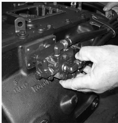
7. Install slave valve and tighten to specifications.
