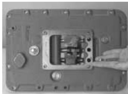
2. Remove the oil trough retaining capscrews and oil trough. (Some models do not have an oil trough.)
