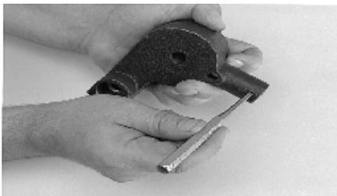
10. From the pump housing, remove the relief valve roll pin.
