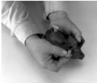
7. Lightly lubricate insert valve O-rings with Eaton® Fuller® Silicone lubricant P/N 71206 or equivalent. Install insert valve with flat side to the inside. Install insert valve retaining nut and torque to 40-50 Lb•ft.
