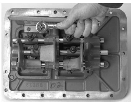
17. Install the shift block and shift yoke lockscREWS, torque to 35-45 lb-ft (47.45-61.01 N•m). Lockwire securely.
