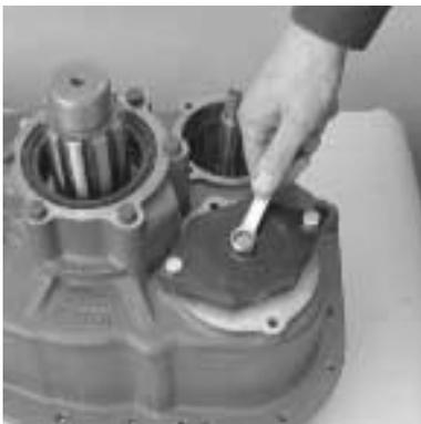
6. Install the assembled outputshaft (see Outputshaft Assembly) between the countershafts and match the timing marks.
