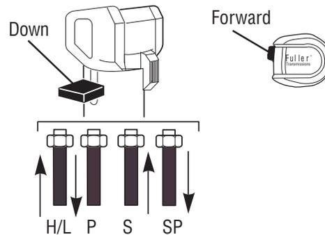
1. A tee fitting on the low range port of the slave valve will supply air through a 5/32" or 1/8" air line to the "H/L" port on the shift knob. Because this line is connected to the low range port, air is only available when low range has been selected.
