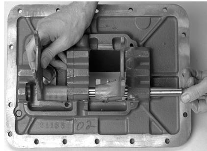
8. Place the actuating plunger in the top center bore.
