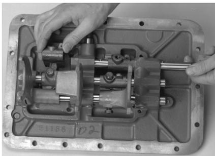
15. Holding the top bar notched-end, start installation. As the bar passes the rear boss, position the shift block.
