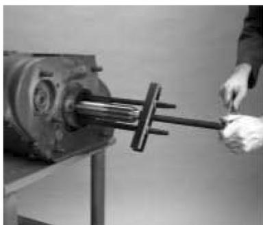
5. Install the bearing puller tool and remove the input bearing from the case and input shaft or use pry bars or screwdrivers to complete removal of the bearing.
