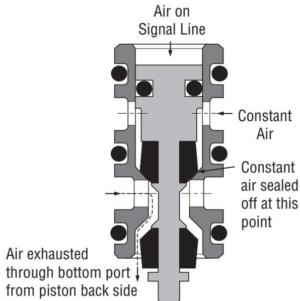
Deep reduction piston moves rearward due to constant air on front side.
