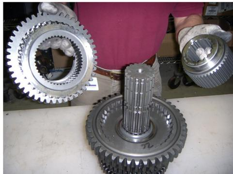
3. Remove the snap ring and key. Mark keyway location.
