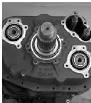
24. Heat rear tapered bearing and install over outputshaft.
