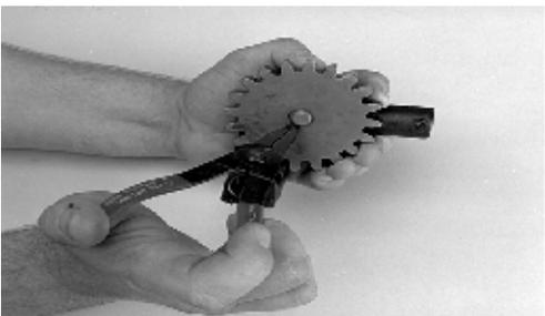
2. From the drive shaft, remove the drive gear retaining snap ring.
