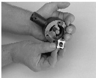
8. Align the inner element keyways with the drive shaft keys and install the integral oil pump inner element.
