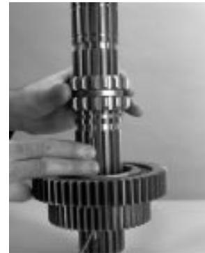
11. Position the next offset washer in the next available groove. Rotate the washer until the washer splines and mainshaft splines align.
