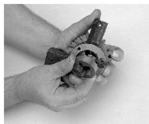
13. Install the outer integral oil pump element over the inner element.
