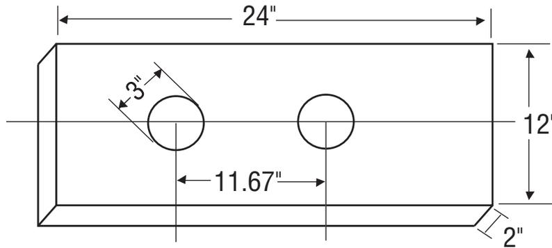
This fixture is designed to ease the assembly of the auxiliary gearing. Set the auxiliary countershaft rear bearings in the 3" holes.
