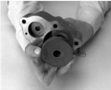
8. Remove the range and reduction pistons from the cylinder bores.
