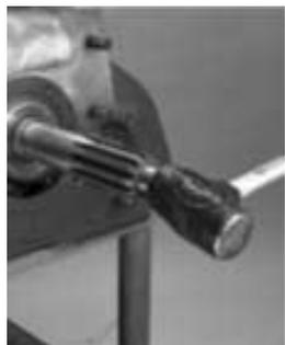
4. Use a soft bar and maul to drive the input shaft toward the case rear as far as possible. Pull the input shaft forward.
