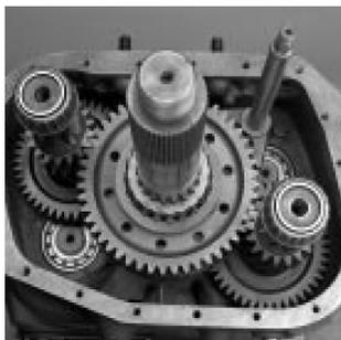
11. Assemble mainshaft assembly into transmission rear. Splines on mainshaft end must slide into range synchronizer. Marked teeth on low a range gear must be aligned with marked teeth on countershafts.
