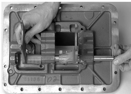
7. From the bottom yoke bar, remove the two (2) shift yokes.
