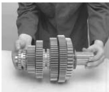
2. Place the mainshaft in a vertical position, pilot end down.
