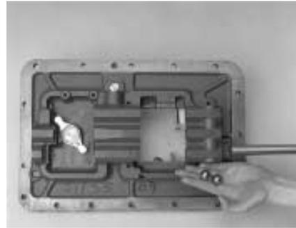
9. If damaged, from the 1st and reverse shift yoke, remove the plug, spring, and plunger.
