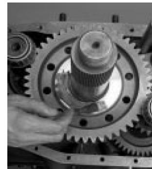
17. Apply grease to reduction gear rear thrust surface.
