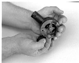
9. Install the inner element retention snap ring in drive shaft snap ring groove.
