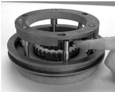
4. Place the HI range synchronizer ring over the LO range synchronizer ring. Rotate the HI range synchronizer until the springs are seated against the pins.
