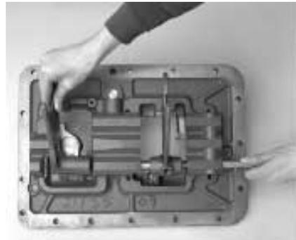
7. Install the shift yoke lockscrew, torque to 35-45 lb-ft (47.45-61.01 N•m). Lockwire securely.
