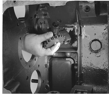
6. Remove the integral oil pump retainer plate from inside the case.
