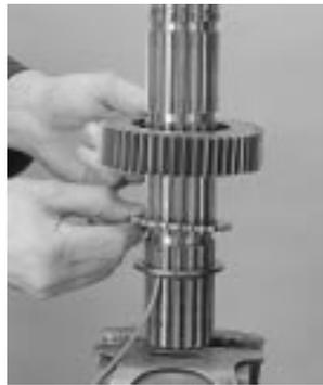
5. Against the 4th speed gear washer, position a spacer washer against the tolerance washer.
