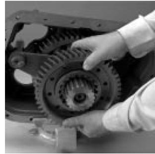
5. From front with a punch and hammer, drive the two coupler pins from the coupler. Align the coupler splines with the washer splines and remove the range coupler from the LO range gear.
