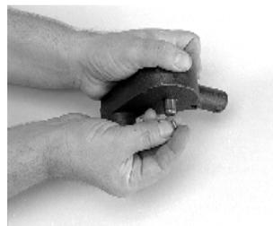
11. Align drive gear keyway with drive shaft key and install the drive gear on the drive shaft.
