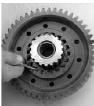
6. Rotate splined washer to align pins and drive pins through lock washer.
