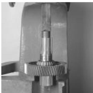
11. Use the reduction gear front face as a base, press the output shaft through the bearing and gear. This frees the bearing, reduction gear, washer, and the splined washer.
