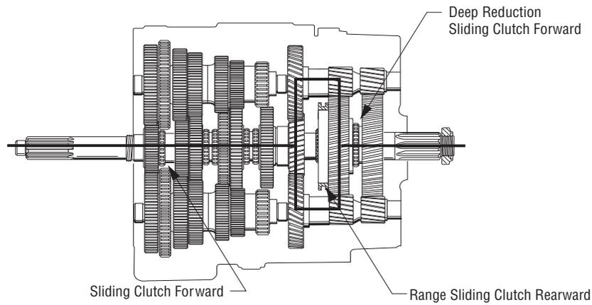
Figure 2-5. Front Section Power Flow - Direct Gear
