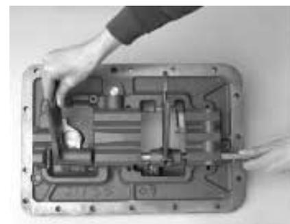
7. From the bottom yoke bar, remove the two (2) shift yokes.
