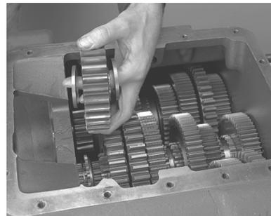
6. Inspect the reverse gear assembly, remove the inner race and needle bearing, if damaged.
