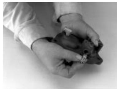
5. Remove the 15/16" nut on the range yoke bar.
