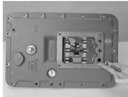
2. Remove the oil trough retaining capscrews and oil trough. (Some models do not have an oil trough.)
