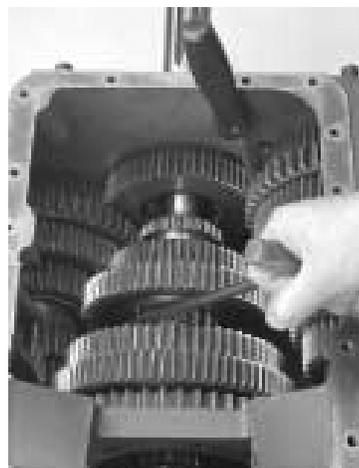
4. Tilt the mainshaft front up and lift the assembly from the case.
