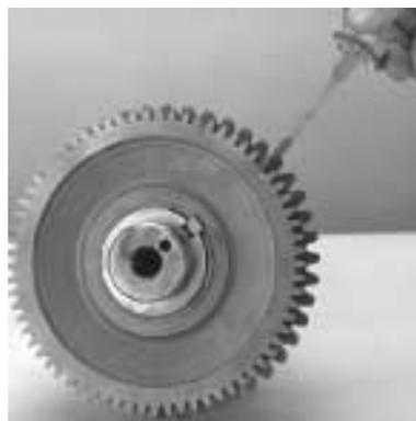
2. Place the lower, 47-tooth PTO gear countershaft, into the main case with the shaft seated in the lower countershaft case bores.
