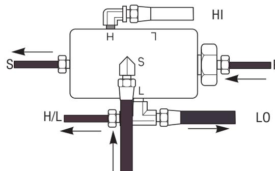
2. When the deep reduction button is moved forward, air from the "H/L" port will pass through the shift knob to the "SP" port. A 1/8" or 5/32" air line connected to the shift knob transfers this air to the insert valve at the deep reduction cylinder cover.
