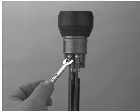
6. Slide the cover into position on the Roadranger valve.
