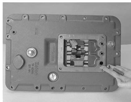
19. Install the three (3) tension balls, one in each housing top bore. Install the three (3) detent springs, one over each tension ball.
