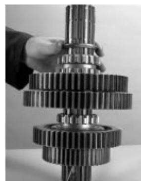
20. From the mainshaft rear, install the mainshaft key into the spline with the air line. Pull the air line from the spline while installing the key.
