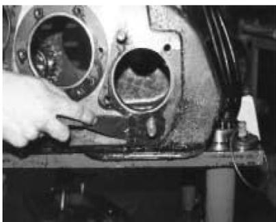
5. Remove the gasket and clean all mounting surfaces of gasket material.
