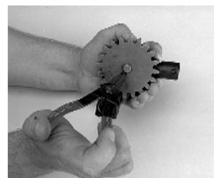
12. Install the outer drive gear retention snap ring in drive shaft groove.
