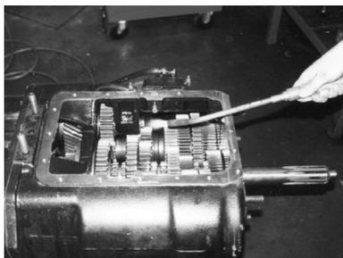
2. The mainshaft reverse gear must be moved in order to remove the upper reverse idler gear. Remove reverse gear snap ring and slide reverse gear forward over clutch.
