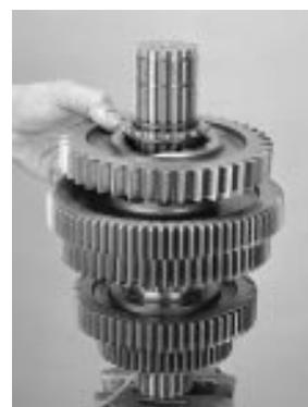
26. At this time remove the air line and insert the mainshaft key. Be careful not to move the gears while doing this procedure, the tolerance washers are unlocked and can rotate which would cause the gears to drop.
