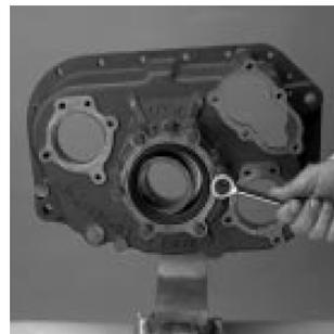
14. Remove the complete bearing race from the bearing bore.
