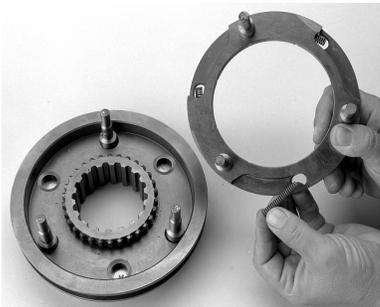
3. In the HI range synchronizer bores, install the three (3) springs.
