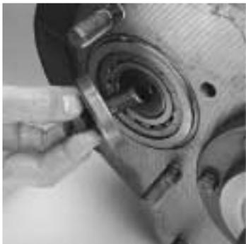
5. From the front of each countershaft, remove the capscrew and front retainer plate.
