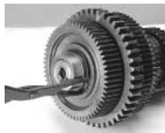
7. Use a flanged-driver or the press to install the bearing inner race on the countershaft front against the drive gear.
