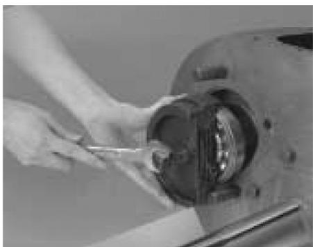
8. Use the appropriate bearing puller T9 or prybars to remove the countershaft front bearings.
