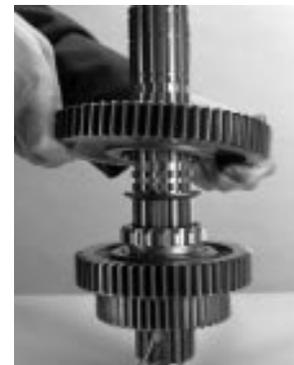
14. Position the flat washer against the gear. Rotate the washer until the washer splines and mainshaft splines align.
