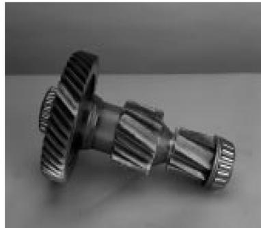
5. Install both countershaft assemblies. Match the timing marks on the auxiliary drive gear with the timing marks on the countershafts.
