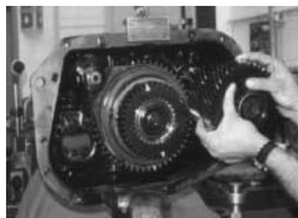
5. Support the auxiliary countershaft while removing the auxiliary countershaft retaining strap.
