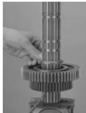
10. Insert two large screwdrivers between the two gears. Apply slight downward pressure to spread the gears evenly. Between the gear hub and mainshaft spacer, insert 0.006" feeler gauge and 0.015" feeler gauge. If out of tolerance, change the washer against the mainshaft spacer.
