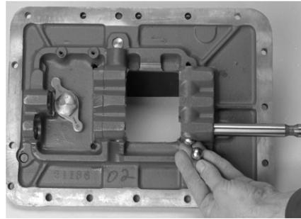
9. If damaged, from the 1st and reverse shift yoke, remove the plug, spring, and plunger.
