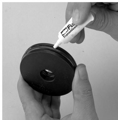
3. Install O-rings onto range and reduction pistons.
