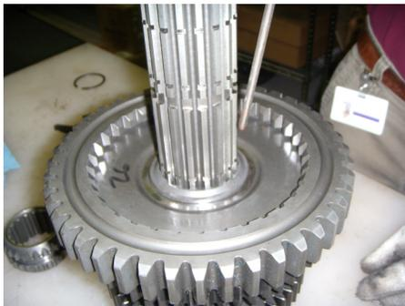
16. Position the offset washer (flat surface down) against the gear. Rotate the washer until the washer splines and mainshaft splines align.
