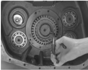
6. Apply Eaton®Fuller® thread sealant #71205 or equivalent to the capscrew threads, and install the six (6) capscrews. Torque the capscrews to 35- 45 Lb•ft. NOTE: On some previous designs, lock wire was used on the capscrews, lock wire as needed.
