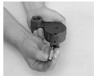
2. Install the relief valve spring in oil pump housing.
