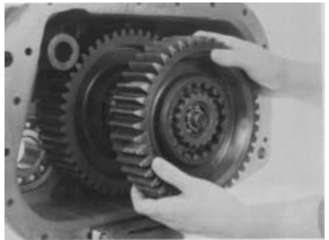
3. Turn the tolerance washer to line up the splines and slide the low range gear off the mainshaft.
