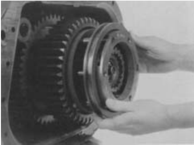
1. Slide the synchronizer from the mainshaft.
