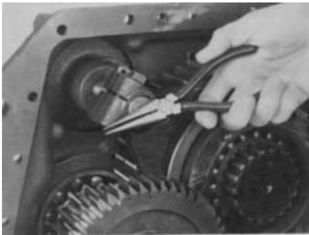
4. Cut the lockwire from the shift yoke cap screws.
