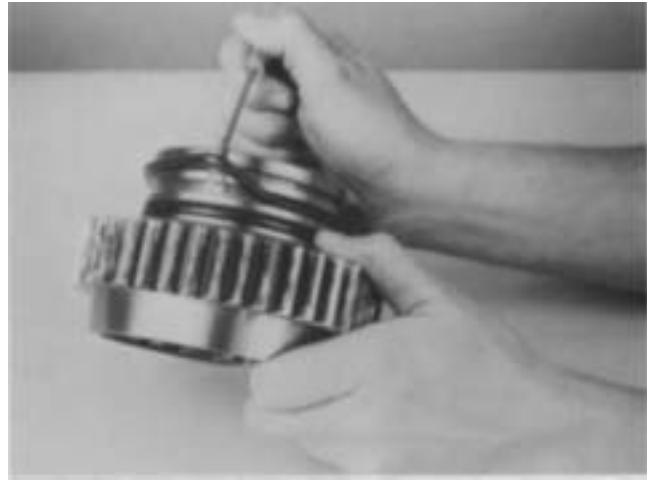
6. If necessary, remove the O-rings from hub O.D. of auxiliary drive gear.
