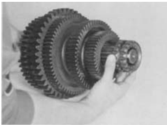
1. Remove the sliding clutch from the mainshaft.
