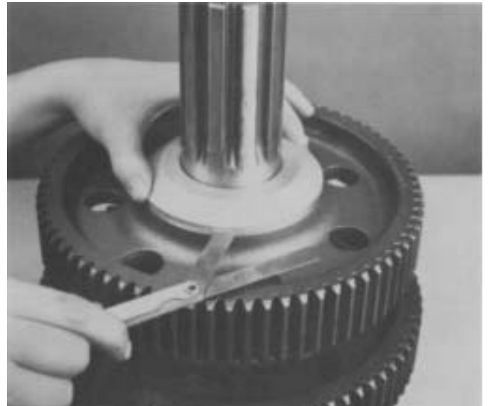
24. Apply downward pressure against spacer and check clearance between spacer and reverse gear with feeler gage. Correct clearance is .005" to .012". If it is necessary to adjust clearance, change tolerance washer in reverse gear.
