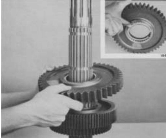
13. Temporarily install snap ring in 2nd speed of gear (inset). Install gear, clutching teeth facing down. Engage clutching teeth of gear with external splines of spacer.
