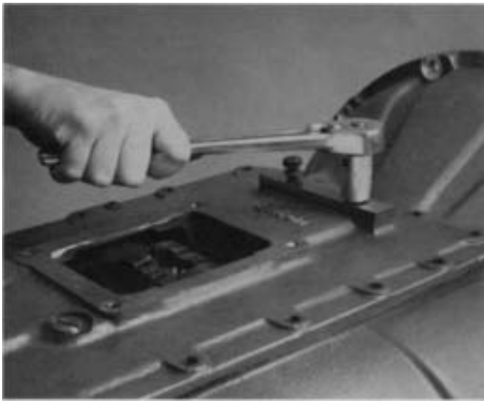
2. Turn out two cap screws and remove tension spring cover.
