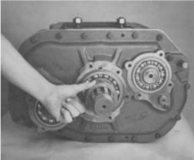
3. Remove spacer from output shaft.
