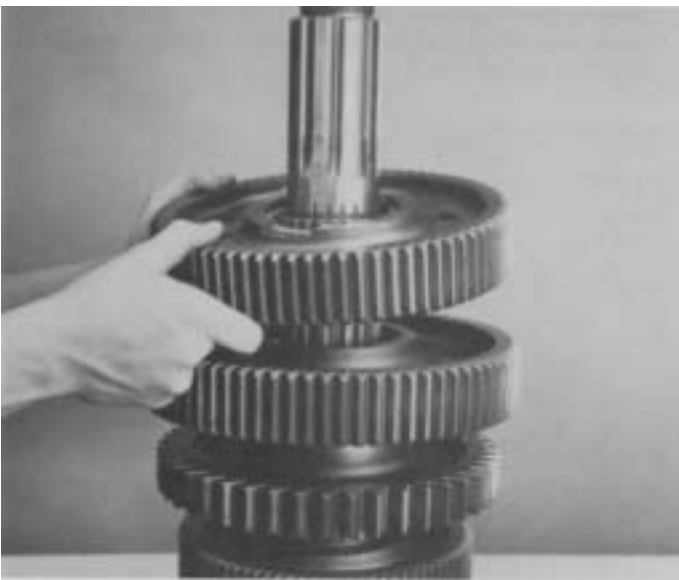
22. Install reverse gear, clutching teeth facing down. Engage clutching teeth of gear with external splines of spacer.
