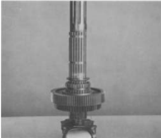
7. Remove mainshaft assembly from vise. Reinstall mainshaft in vise with pilot of mainshaft facing down.
