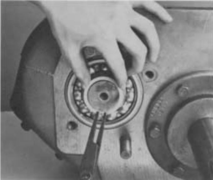
13. Remove snap rings from the front of both countershaft.
