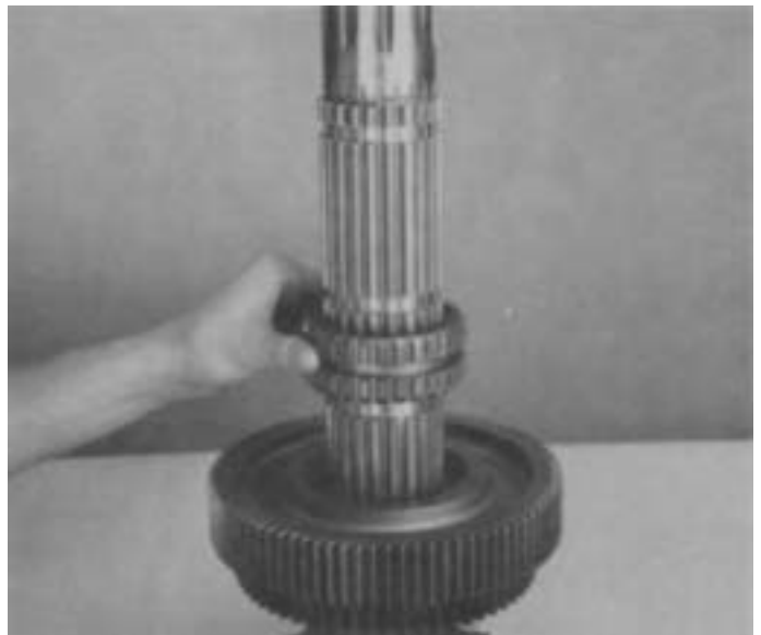
9. Remove 2nd and 3rd speed clutch from rear of mainshaft.
