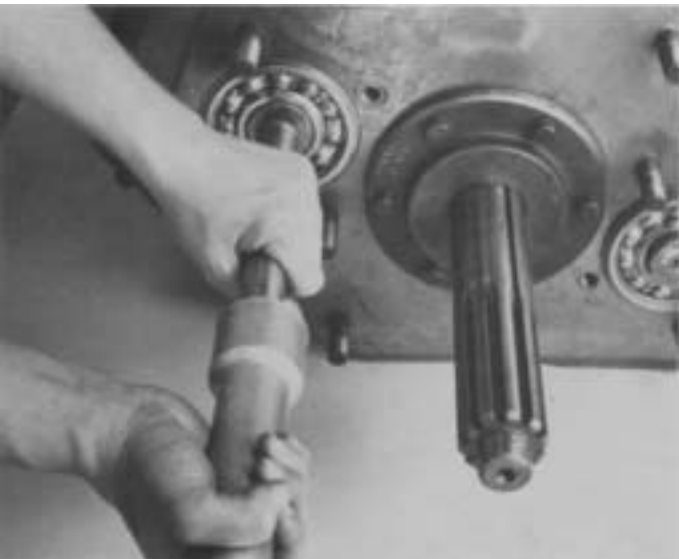
14. With soft bar and maul drive right countershaft to rear until front of countershaft is even with front of bearing.
