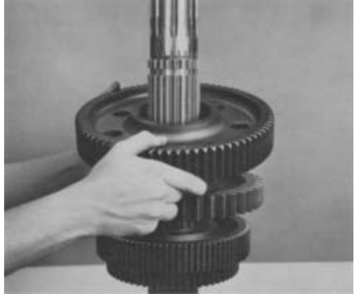
15. Install 1st speed gear with clutching teeth facing
