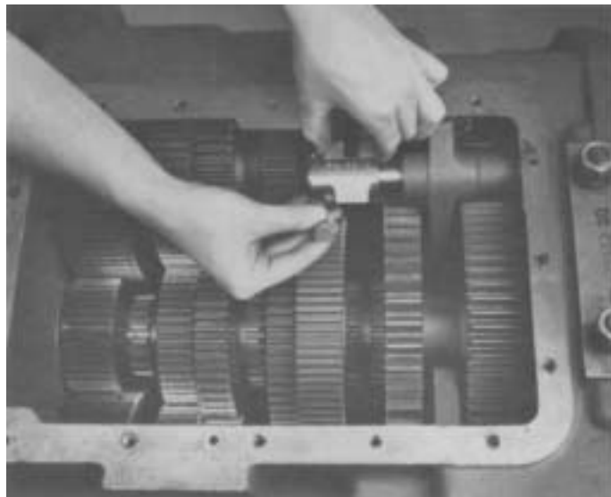
3. Cut lockwire, remove cap screw and 1st/reverse block.
