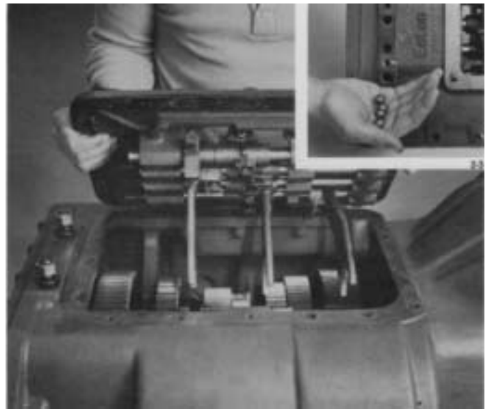
4. Jar housing lightly to break gasket seal and lift housing from transmission. Tip housing over to remove four balls in tension spring bores (inset).
