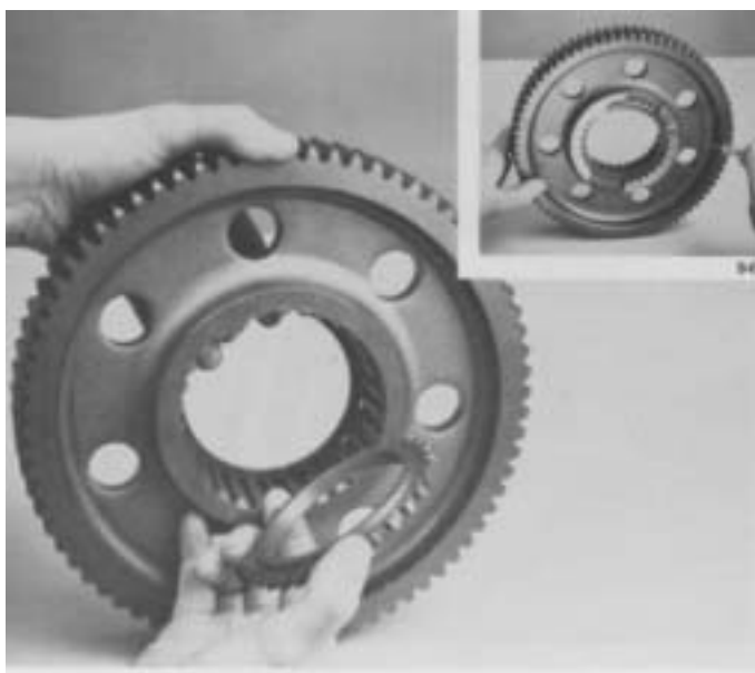
2. Remove washer from hub of reverse gear and snap ring from reverse gear if necessary (inset).
