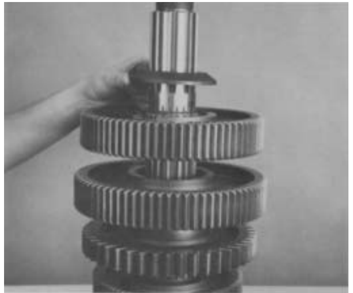
23. Install washer, with tapered side facing up, against reverse gear.
