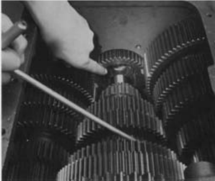
37. Lower pilot end of mainshaft into position with pocket bushing of input shaft.
