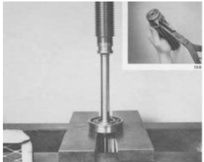
5. Block the countershaft bearings and press them from shaft, remove inner snap ring (inset) if so equipped.
