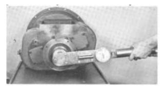
spacer of the same width must be used. Failure to pull the yoke or flange tightly into place will permit the shaft to move axially with resultant damage to rear bearing.
